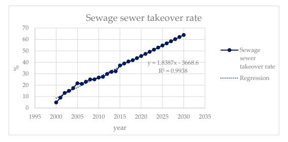
Figure 15. Estimated trend of the sewage sewer takeover rate from 2000 to 2030 [58].
