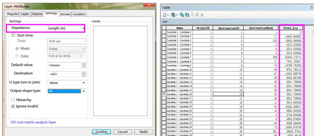
Figure 7. Set the origin–destination (OD) cost matrix parameter and output the spatial distance.
