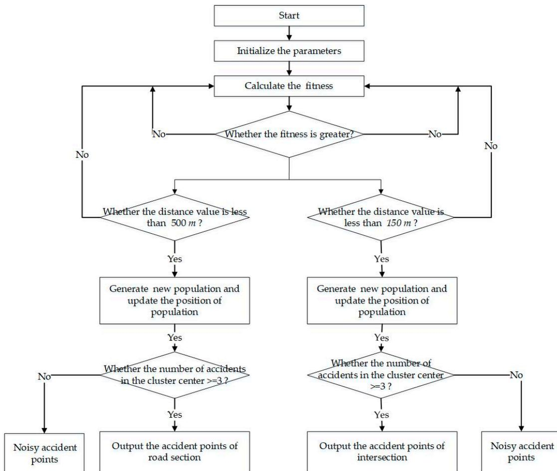
Figure 4. Flowchart of the Firefly Clustering Algorithm.
