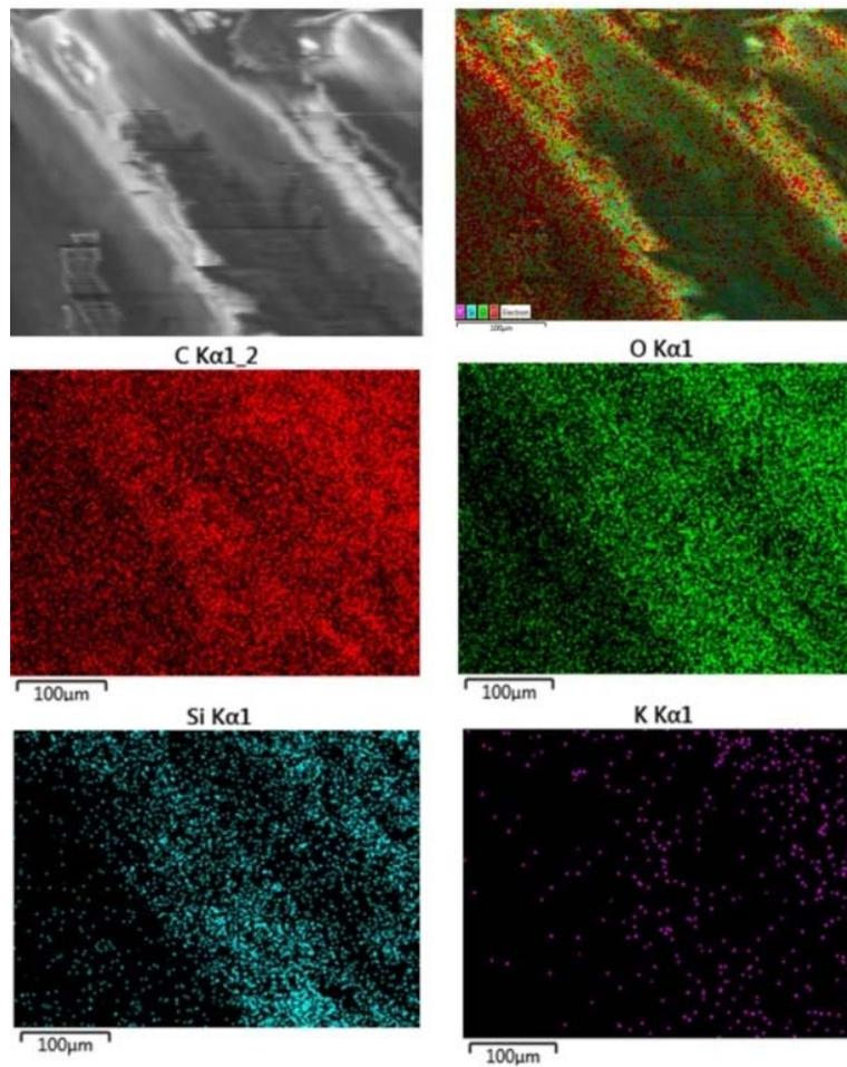
Figure 9. Mapping analysis of elements in wheat straw WH-1105.
