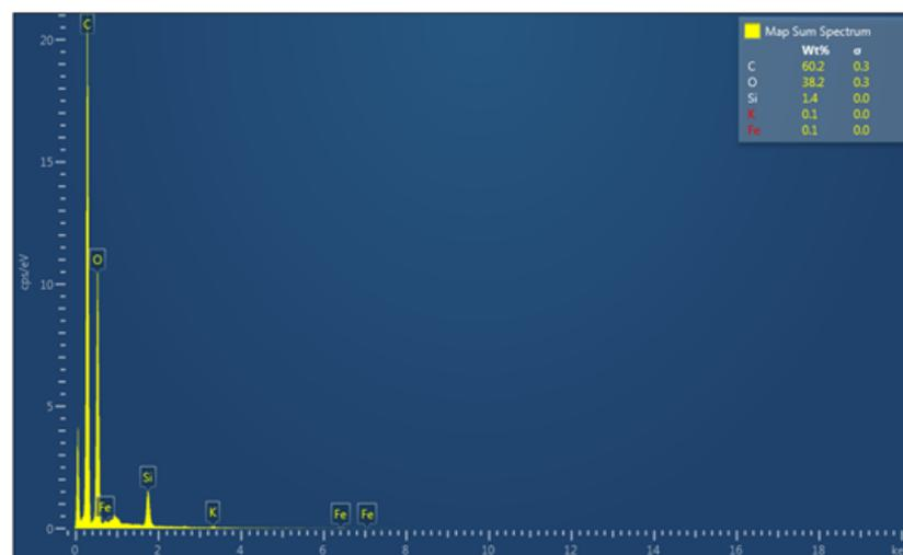
**Figure 8.** Energy dispersive spectroscopy of wheat straw WH-1105.
