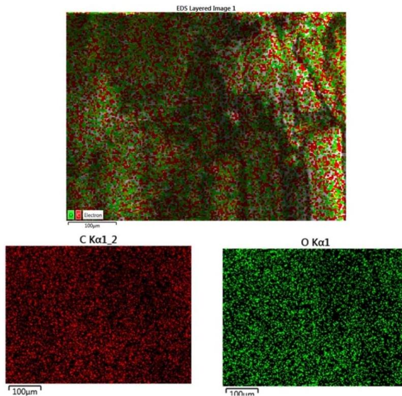
Figure 11. Mapping analysis of elements in wheat straw HD-2967.
