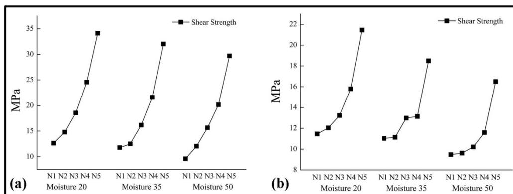
**Figure 5.** Variation in shear strength with respect to moisture (%) and nodes in (a) variety WH-1105 and (b) variety HD-2967.
