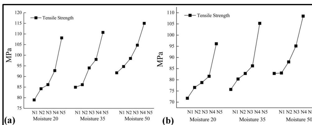
**Figure 4.** Variation in tensile strength with respect to moisture (%) and nodes in (a) variety WH-1105 and (b) variety HD-2967.
