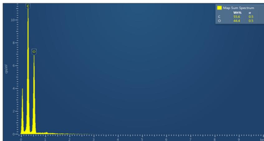
Figure 10. Energy dispersive spectroscopy of wheat straw HD-2967.
