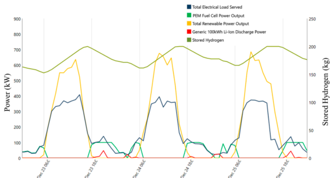
Figure 7. The stand-alone microgrid (SAM) system components' operations of S3 hybrid system (December).
