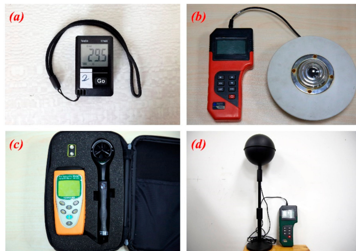
Figure 6. Photographs of instruments for meteorological measurements: (a) mini temperature and humidity recorder, (b) solar radiometer, (c) anemometer, and (d) black globe thermometer.
