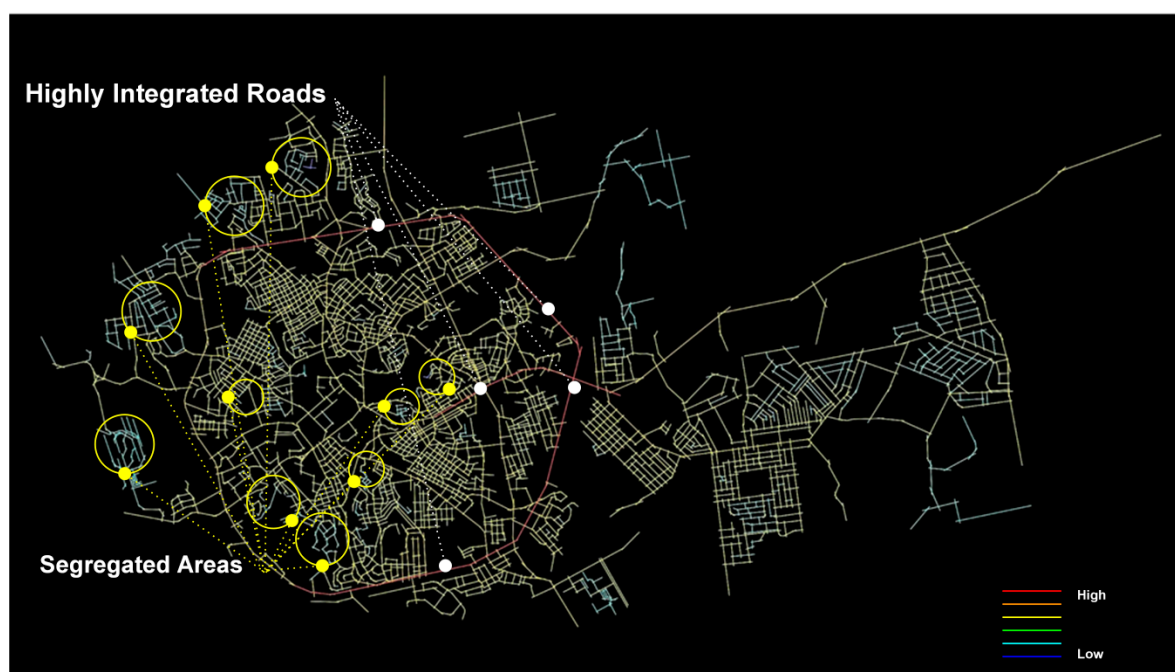
Figure 6. Angular Segment Analysis_T1024_Integration_Rn (Global), (Generated using Depthmap).
