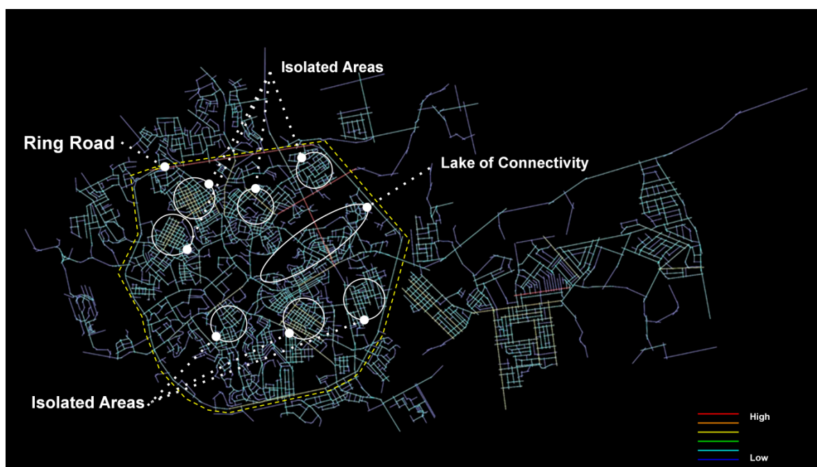
Figure 5. Angular Segment Analysis_T1024 Choice_R1200, (Generated using Depthmap).
