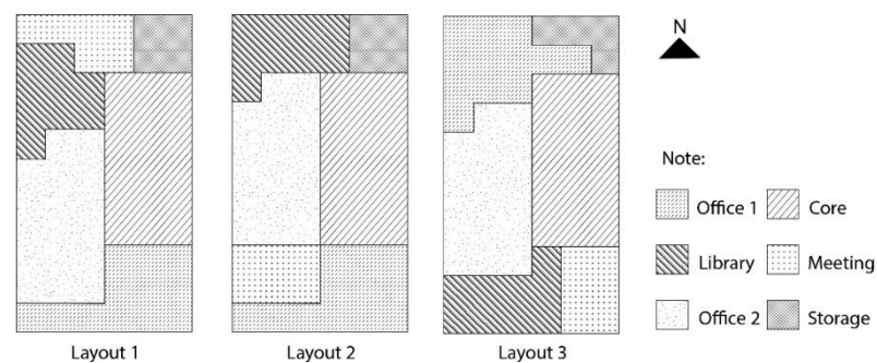
Figure 7. Three layouts with similar WWRs in [68]. The interior partitions divide the layout into different thermal zones.
