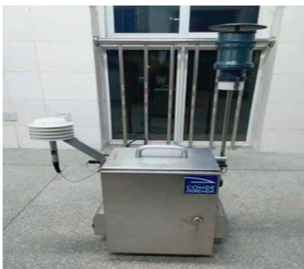
Figure 3. COMDE DERENDA particulate sampler.
