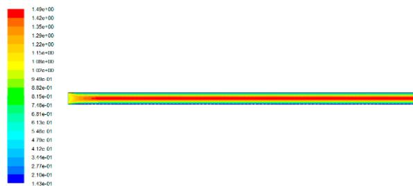
Figure 22. Velocity vector ( $\Delta P = 7 \text{ pa}$ ).
