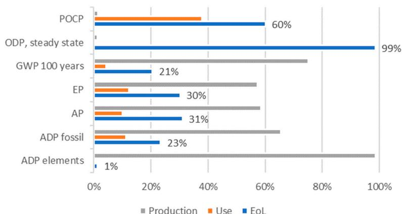
**Figure 6.** Relative contributions of phases (production, use, EoL) for assessment of the construction with recycled brick aggregate in case of the scenario with reuse of blocks (Plan 1 s2) (all indicators, %), according to CML2001.
