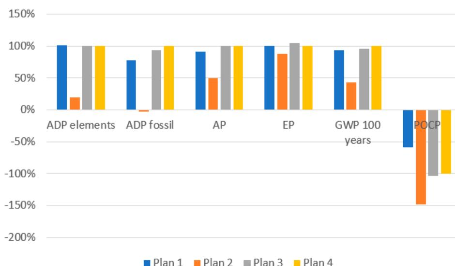
**Figure 3.** Relative comparison of assessed blocks in the scenario with 50-year-long life span, the reusability was not considered (scenario 1) [%], the result of Plan 4 is 100%, except the ODP indicator].
