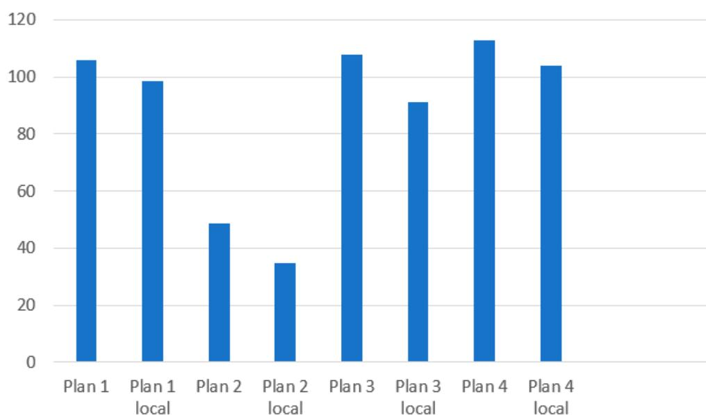
**Figure 8.** Comparison of local transport (distance parameter is 50 km) and default transport (distance parameter 100 km) in scenario 1, impact in Global Warming Potential (GWP 100 years) (kg CO<sub>2</sub> eq.), according to CML2001.
