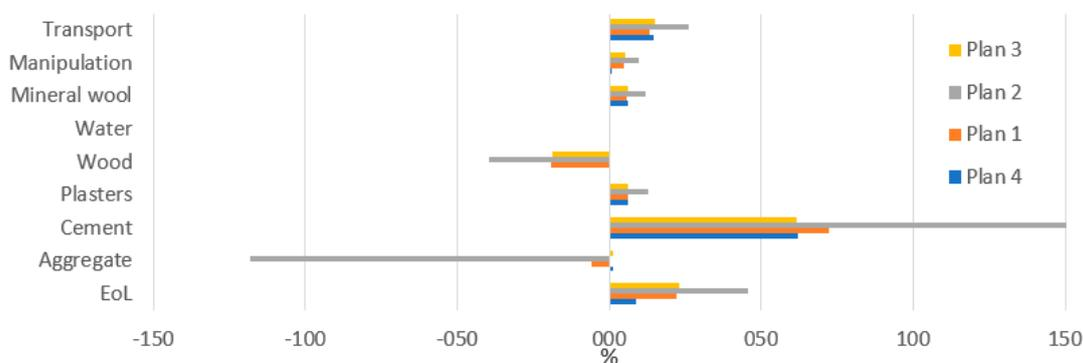
**Figure 5.** Relative contributions of processes related to the whole impact of plans in the scenario with 50-year-long life span, the reusability was not considered (scenario 1) (for GWP indicator, %), according to CML2001.
