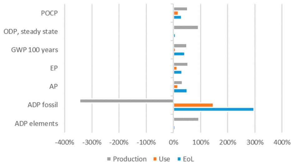
**Figure 7.** Relative contributions of phases (production, use, EoL) for assessment of the construction with recycled concrete aggregate in case of the scenario with reuse of blocks (Plan 2 s2) (all indicators, %), according to CML2001.
