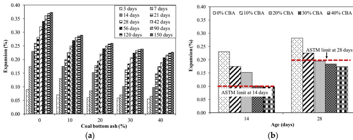
**Figure 10.** Expansion results and ASTM limits for mixture with various proportions of CBA. (a) Expansion results, and (b) ASTM limits for expansion.
