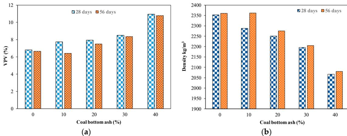
**Figure 4.** Volume of permeable voids (VPV) and density results at various ages. (a) VPV for mixtures with CBA, and (b) density for mixtures with CBA.
