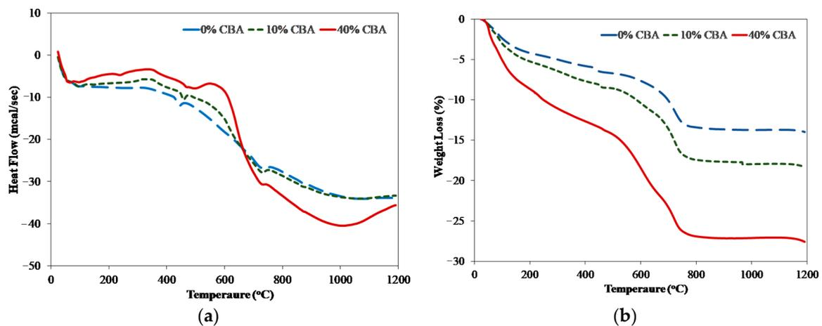
Figure 6. Thermal analysis of specimens incorporating various proportions of CBA. (a) Heat flow, and (b) Weight loss.
