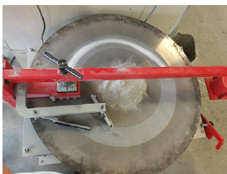
Figure 3. Böhm's device for determining the resistance of concrete to mechanical abrasion.
