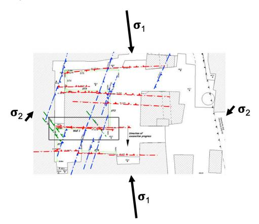
**Figure 4.** Map of the northwestern chamber of the Ravaccione quarry with the indication of the main surveyed discontinuities (red, blue, and dark green dashed lines) and the principal stress components measured using CSIRO cells ( $\sigma_3$  is not reported because it is normal to the other stress components). The rectangular shape shows the location of the survey (modified after [7]).
