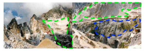
**Figure 14.** Carrara marble quarry basin: open pits and *Ravaneti* (green dashed lines). Some of the historical *Ravaneti* (blue dashed line) have been used as a base for the internal roads in quarrying areas.
