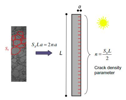
Figure 12. Scheme of the intergranular equivalent cracking (after [20]).
