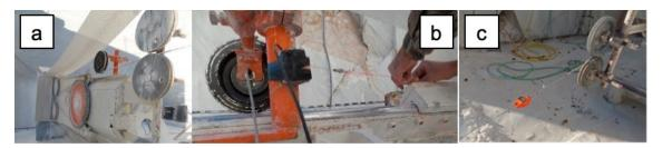
**Figure 7.** (**a**) Positioning of the load cell on the Apuania Corsi MF 5000 machine. (**b**) Placing the draw wire encoder. (**c**) Installing the dynamometer for calibration.
