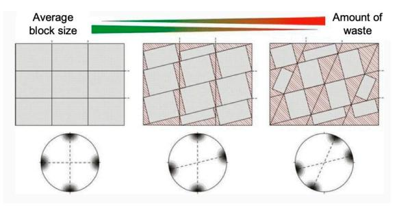
**Figure 2.** The amount of waste increases while the average extractable block size decreases due to the joint system deviating from orthogonality where the spacing pattern remains equal. The characteristic joint density distributions depict the orientations of each joint pattern (modified from [41]).
