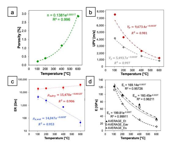
**Figure 10.** Relationship between (**a**) the average porosity, (**b**) the average P- and S-wave velocity, (**c**) the average dry and wet average electrical resistivities, and (**d**) the average values of Young's moduli of marble samples and the temperature to which the samples had been exposed.
