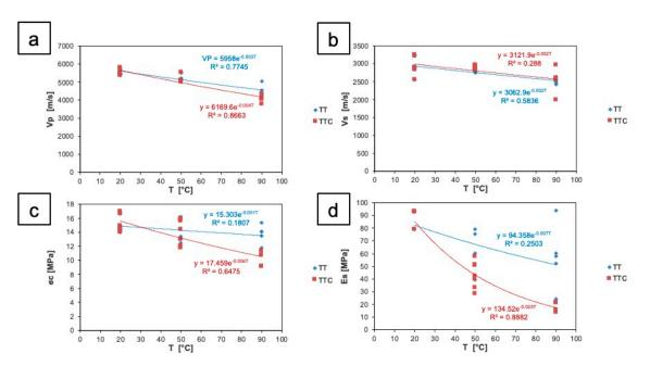
**Figure 11.** Relationship between (**a**) P-wave velocity, (**b**) S-wave velocity, (**c**) Shear resistance, and (**d**) secant Young's moduli as a function of temperature for Carrara marble sample after thermal (TT) and coupled thermo-chemical treatment (TTC).
