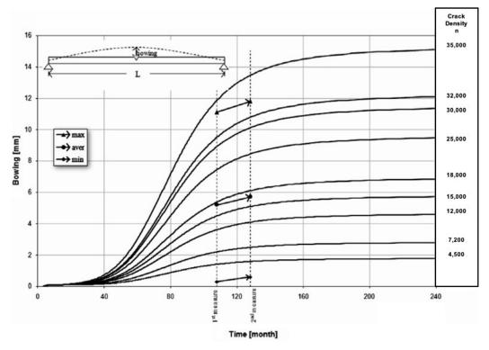
**Figure 13.** Total (bulk and crack-induced) deflection as a function of the number (expressed in months) of thermal cycles for the simply supported slab with different values of crack density n (after [20]).
