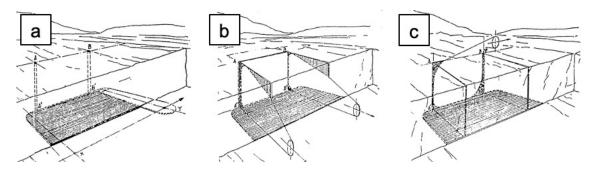
**Figure 9.** Cooperation between a diamond wire cutting machine and chain cutting machine. (**a**) Drilling of the vertical holes for the loop closure of the diamond wire. (**b**) Horizontal cut at the bottom of the bench through a chain saw (thickness of the cut: about 37 mm, enough to allow the passage of the wire circuit). (**c**) Cutting of the side surfaces and the rear surface using a diamond wire cutter.
