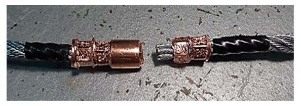
Figure 5. Breakage of the connector clamp, close of the variation in the resistant cross-section.
