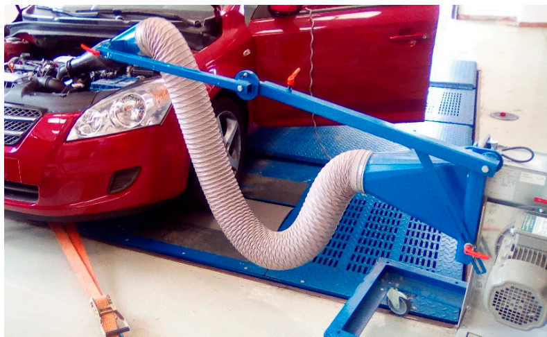
Figure 5. Attachment of ventilator in front of the throttle.
