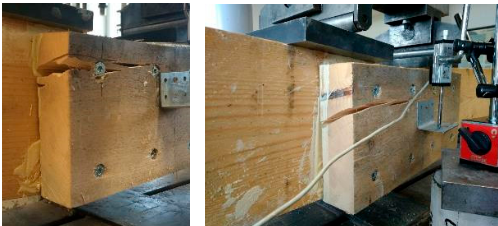
Figure 13. Combination of gluing and screws with solid timber splice: typical failures of solid timber splice.
