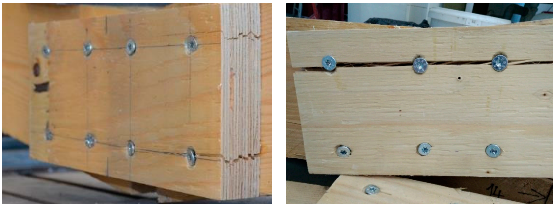
Figure 9. Screw joints with LVL splice: typical failures.
