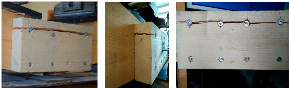
Figure 10. Screw joints with solid timber splice: typical failure of solid timber splice.
