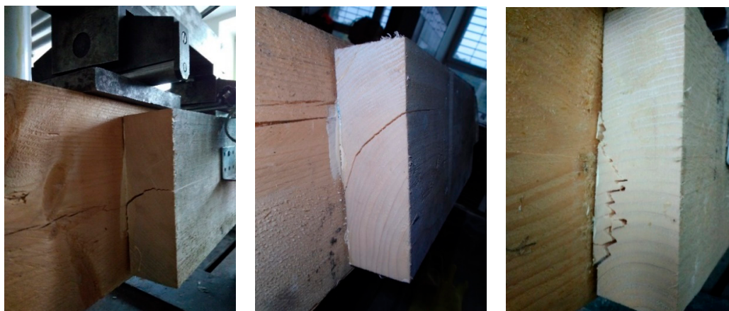
Figure 7. Glued joints with solid timber splice: typical failure of solid timber splice.
