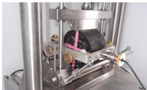
Figure 4. Resilient modulus test equipment.
