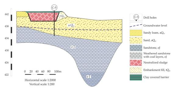
Figure 2. Cross-section through the reservoir (storage).
