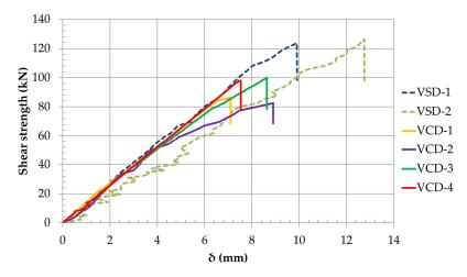
Figure 10. Shear strength–displacement curves.
