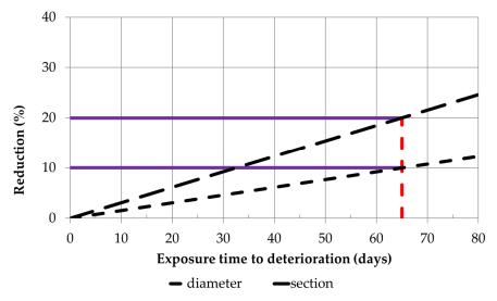
**Figure 1.** Loss of diameter and cross-section per time.  $\theta_i = 8$  mm,  $i_{corr} = 200 \mu A/cm^2$ .
