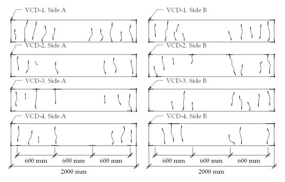
Figure 12. Cracking patterns of severe corrosion at the locations of the shear reinforcements.
