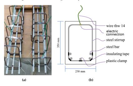
**Figure 3.** Assembly preparation for deterioration induction. (a) The reinforcement of the beam and its connections before being cast; (b) a diagram of the beam with details of connections for corrosion induction.
