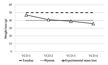
Figure 14. Ratio of experimental and calculated mass loss.
