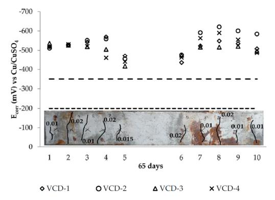
Figure 13. Electrochemical values at the locations of the shear reinforcements.
