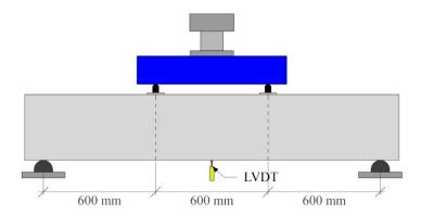
Figure 5. Testing scheme. LVDT: linear variable displacement transducer.
