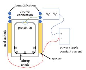
Figure 4. System for application of current, humidification and drying.
