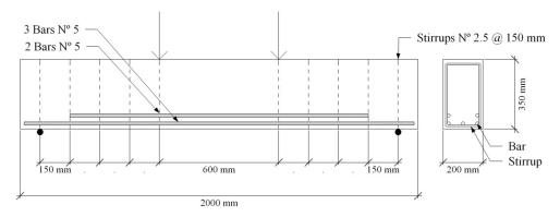
**Figure 2.** Structural arrangement to promote shear failure.
