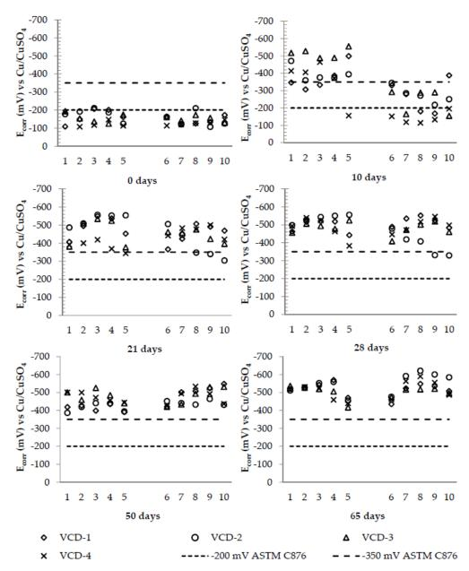
Figure 8. Electrochemical monitoring by measuring the corrosion potentials in the stirrups.
