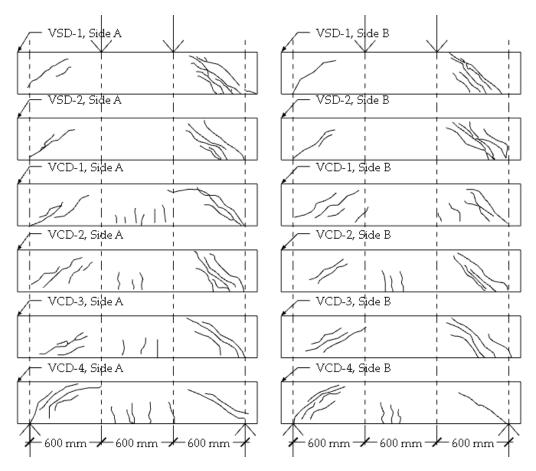
Figure 11. Cracking patterns obtained during the shear tests.
