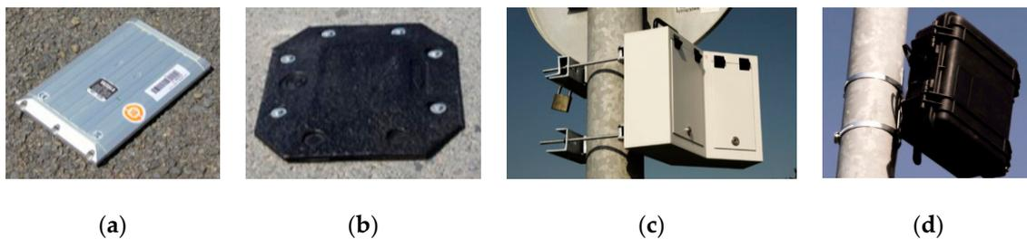
**Figure 2.** Automatic counter devices for measurement of traffic intensity: (a) NU-METRICS NC-200 counting cards; (b) special cover for NC-200; (c) VIACOUNT II counter device; (d) ICOMS-TMS-SA counter device.
