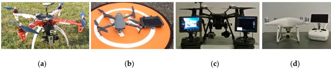
**Figure 8.** Used types of unmanned aerial vehicle (UAV): (a) DJI F450 quadcopter, (b) MAVIC 2 ZOOM, (c) DJI Matrice 210 RTK, (d) Phantom 4 Pro V2.
