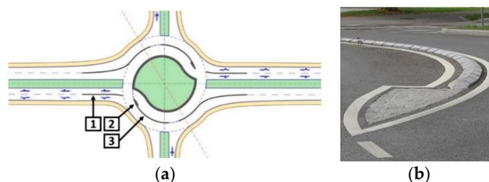
**Figure 1.** (a) An example of the chosen type of turbo-roundabout; (b) an example of the physical separation of lanes on a circulatory roadway (3), including a spike (2).
