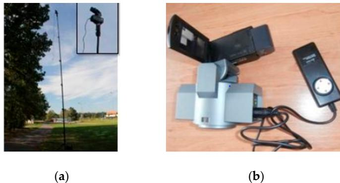
**Figure 4.** Use of a seven-meter tripod (a) with a rotating head (b).
