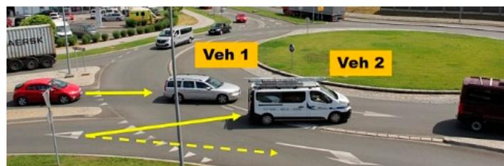
**Figure 16.** Dangerous approach to the turbo-roundabout: there is a subsequent crossing of the paths of the vehicles (Koper, Slovenia; GPS: 45.5451967 N, 13.7447347 E).
