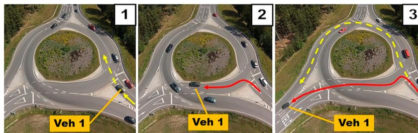
**Figure 18.** Driving in the opposite direction: dangerous entrance of the vehicle in the opposite direction (Jihlava, Czech Republic; GPS: 49.3809189 N, 15.5125189 E); (1)–(3): successive phases of traffic conflict.
