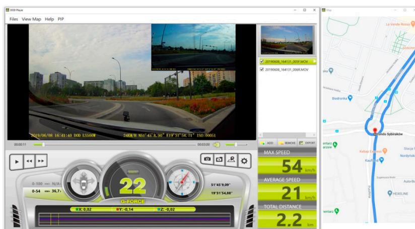
**Figure 6.** Fitting of video cameras in the so-called floating vehicle and the display of operating data in the DOD Player program.
