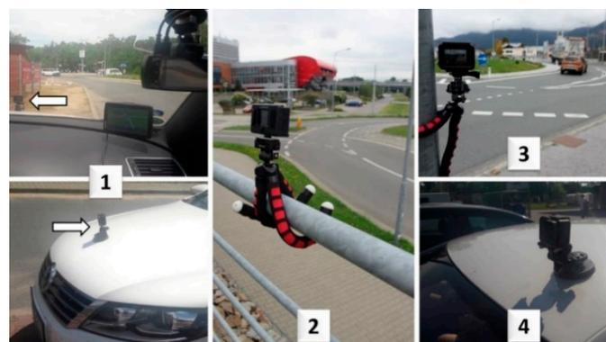
**Figure 5.** Examples of installations of special outdoor cameras for measurements at turbo-roundabouts ((1): position on the front of the vehicle; (2): use of a railing; (3): use of a public lighting pole; (4): position on the roof of the vehicle).
