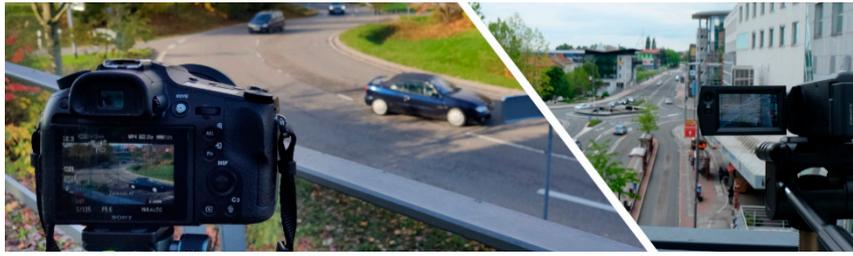
**Figure 3.** Examples of recording devices: Sony DSC-RX10 III camera on the left; Sony HDR-CX450 video camera on the right.
