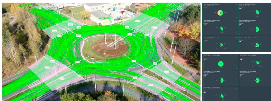
**Figure 9.** Example from the web interface of the program while working in the GOODVISION program (vehicle tracks are marked in green on the left, and graphs for individual directions are shown on the right).
