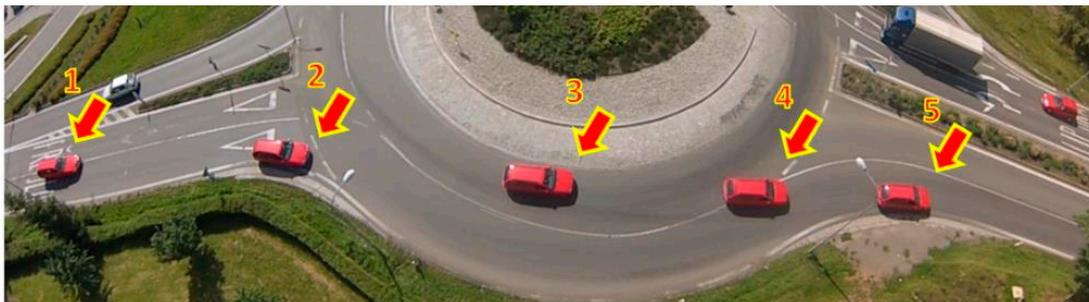
**Figure 12.** Not respecting traffic signs: direct passage via the turbo-roundabout (Olomouc, Czech Republic; GPS: 49.5890953 N, 17.3134856 E); (1)–(5): successive phases of the traffic conflict.
