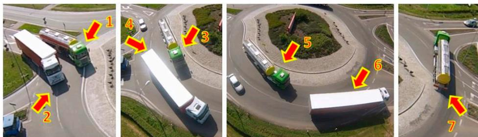
**Figure 14.** Unwanted guidance of vehicles: there is a subsequent crossing of the paths of the vehicles (Olomouc, Czech Republic; GPS: 49.5890953 N, 17.3134856 E); (1)–(7): successive phases of traffic conflict.
