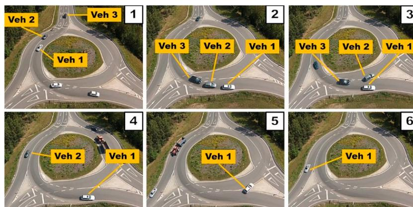
**Figure 20.** Stopping of the vehicle on the circulatory roadway (Jihlava, Czech Republic; GPS: 49.3809189 N, 15.5125189 E); (1)–(6): successive phases of traffic conflict.
