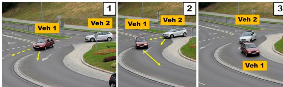
**Figure 15.** Unwanted shortening of the driving path: crossing from the outer to the inner lane at the point of entering the turbo-roundabout (Maribor, Slovenia; GPS: 46.5510875 N, 15.6498817 E); (1)–(3): successive phases of traffic conflict.
