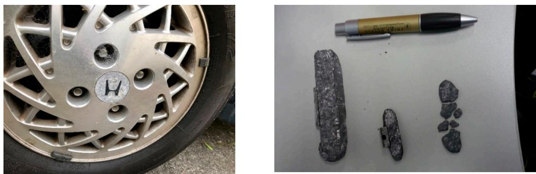
**Figure 1.** Tyre weights clipped to the rim of a wheel and weights collected from the road.
