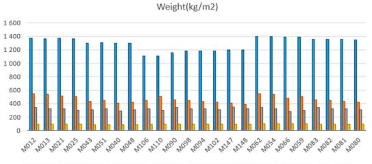
■ CONCRETE AND CEMENTS ■ CERAMIC AND BRICK ■ AGGREGATES AND STONES ■ METALS AND ALLOYS **Figure 4.** Weight per floor area (kg/m<sup>2</sup>) of families of materials (Romania).
