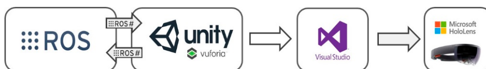
Figure 6. Design of augmented reality application with HoloLens.
