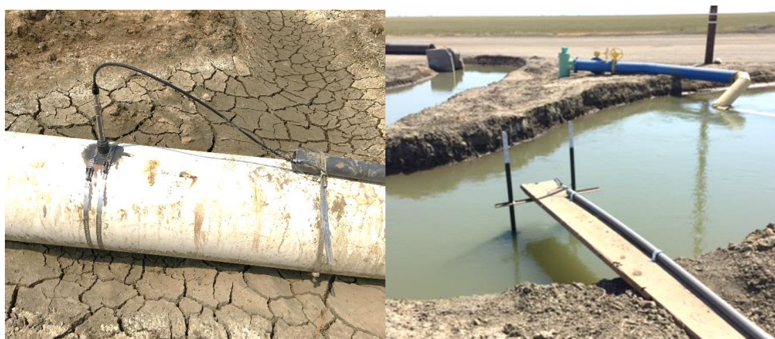
Figure 3. EC sondes installed at each field inlet for the real time monitoring of the salinity and water depth in the supply ditch. The daily irrigation application volumes were supplied by the water master at Panoche Water District. The images show the supply ditch and gated pipe installations of the In-Situ sondes, which are capable of reading EC, temperature and pressure (the depth of the water in the ditch).
