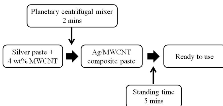
**Figure 2.** The preparation process of Ag/MWCNT pastes.
