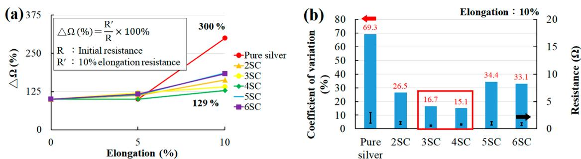
**Figure 8.** (a) The effects of tensile elongation and hybrid paste formulation on the changing percentage of the electrical resistance of PTFE/Ag/MWCNT conductive films and (b) the coefficient variance of the electrical resistance of PTFE/Ag/MWCNT film under 10% tensile elongation.
