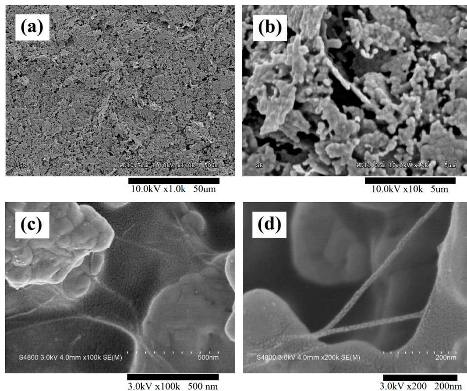
**Figure 5.** VVSEM images of the Ag/MWCNT conductive circuit in sample 4SC. (a) Topography, (b) morphology and arrangement of the silver flakes, (c,d) connections between the MWCNTs and silver flakes.
