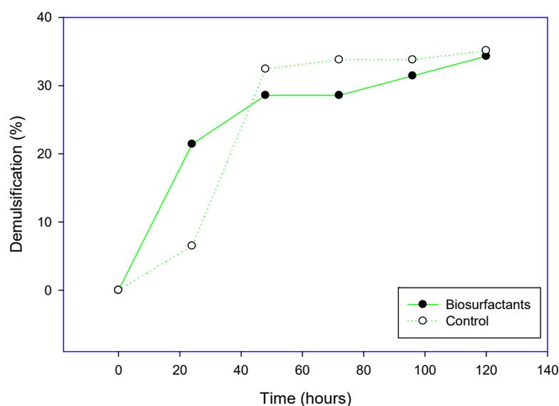
**Figure S2:** Demulsification effect of the biosurfactant supernatant on O/W emulsions of Tween-Triton-Kerosene
