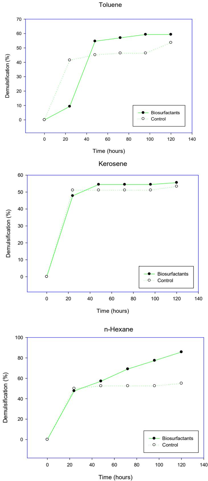
**Figure S1.** Demulsification effect of the biosurfactant supernatant on W/O emulsions of Toluene, Kerosene and n-Hexane.
