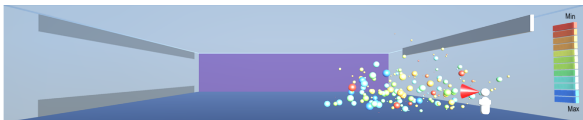
Figure 9. Initially the larger and smaller droplets are in seemingly random positions and random heights.
