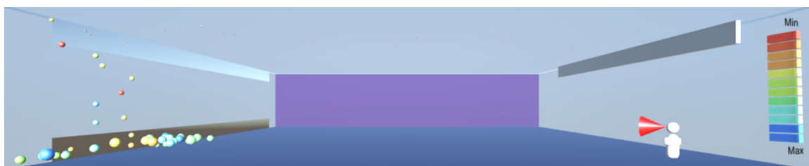
Figure 18. Air vents are opened and the droplets are gradually expelled from the room under the uniform air velocity in the x direction.
