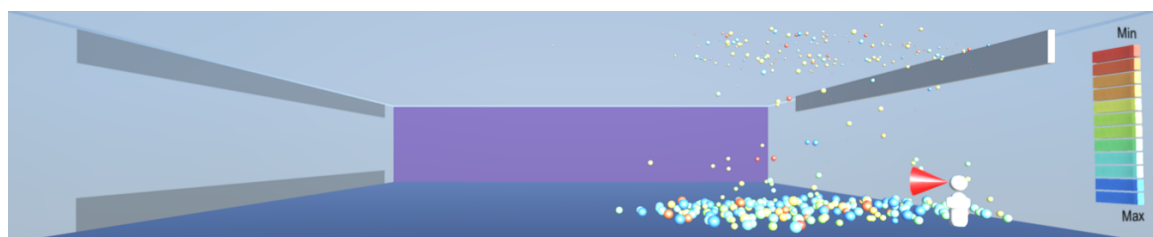
Figure 20. The combined droplets stratify so that larger particles settle near the floor and smaller particles rise towards the ceiling.
