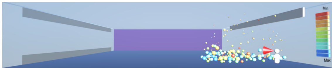
Figure 11. The droplets are ejected into the room to investigate the effect of random air velocities.
