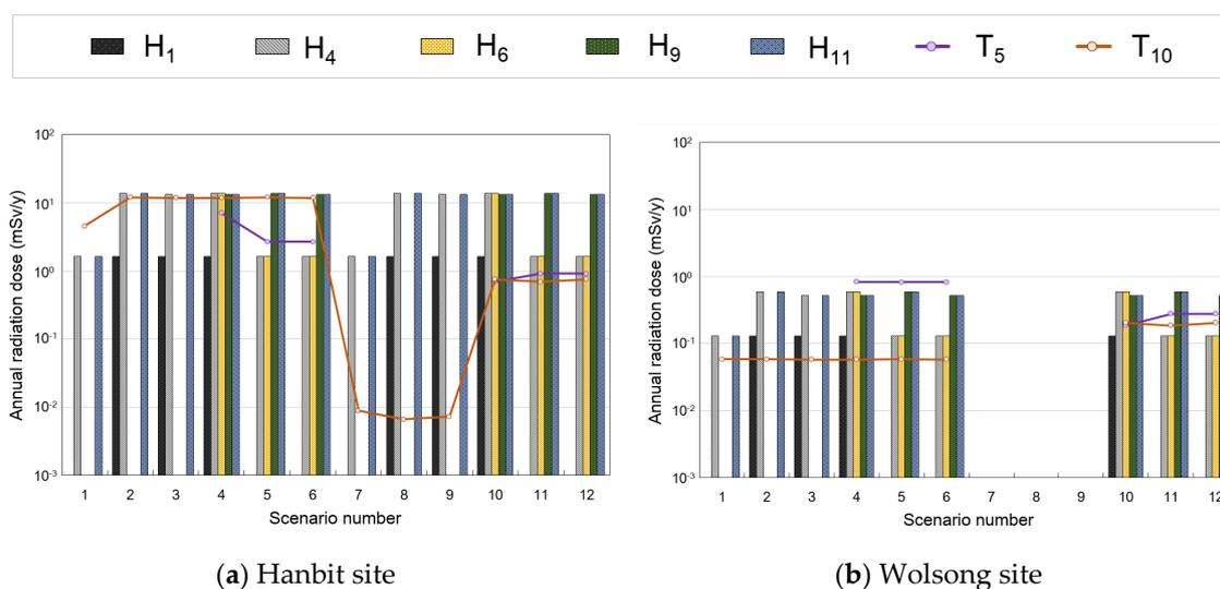
**Figure 6.** Calculated radiation dose of the receptors T1–T3 and H involved in the transportation of the steam generators from two NPP sites.
