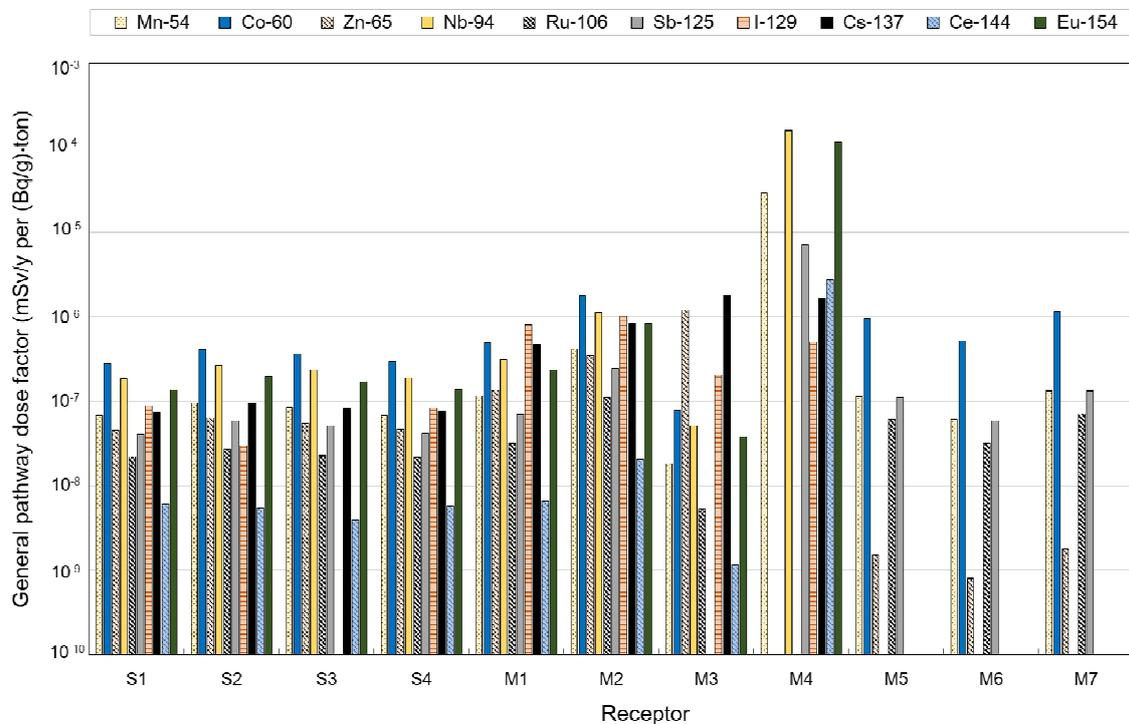
**Figure 3.** General pathway dose factor calculated in this study for each non-actinide and for each receptor in the processing of a steam generator.
