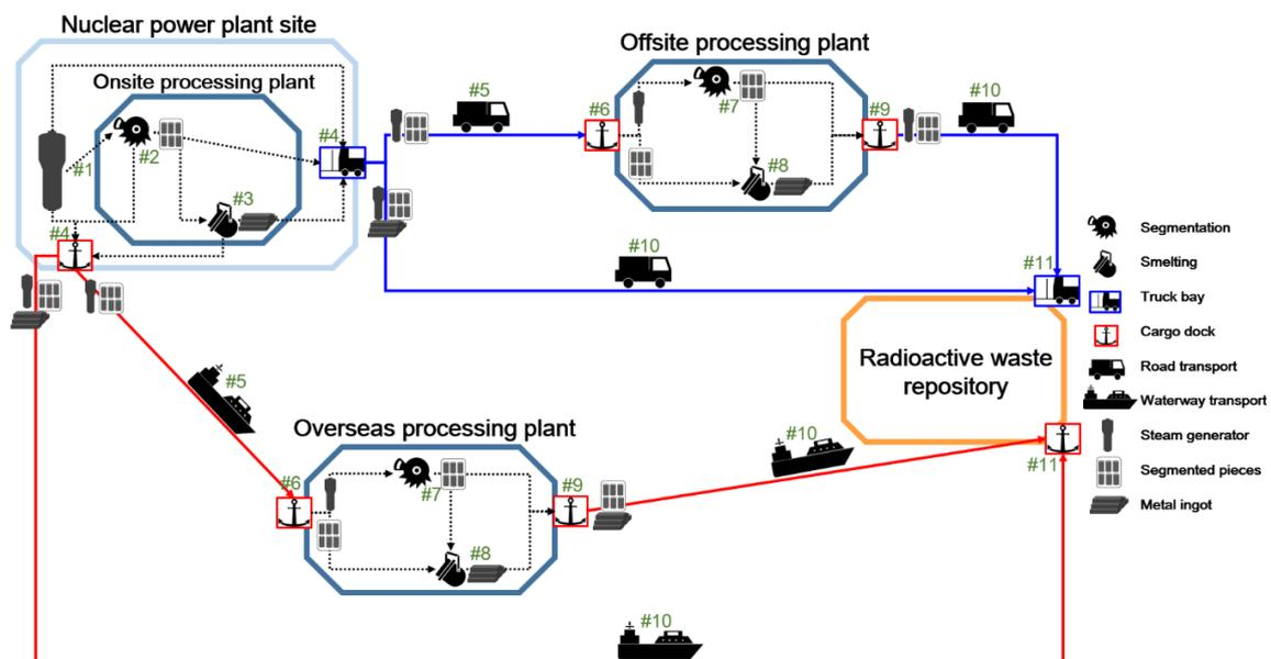
**Figure 1.** Schematic view of the generalized potential scenarios and the respective locations for the predisposal management of steam generators from nuclear power plants.
