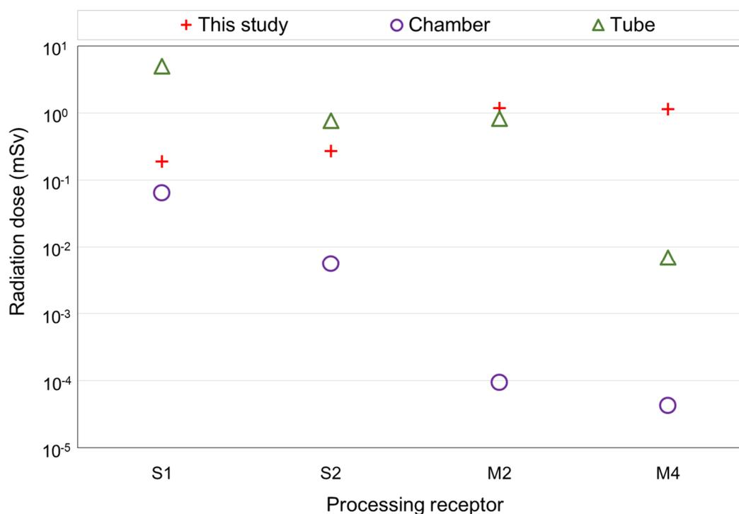
**Figure 7.** Comparison of the radiation doses for the receptors  $S_1$ ,  $S_2$ ,  $M_2$ , and  $M_4$  calculated in this study and presented in the comparable reference study [14]. Plots for the “Camber” and “Tube” represent the estimated radiation doses for the workers processing the chambers and tubes of the steam generator, respectively, in the reference study.
