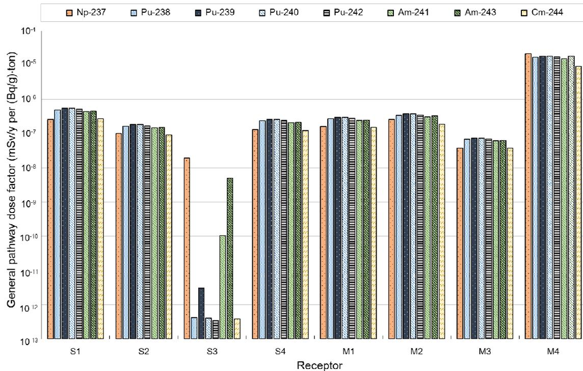
**Figure 2.** General pathway dose factor for each actinide and for each receptor in the processing of a steam generator as calculated in this study.
