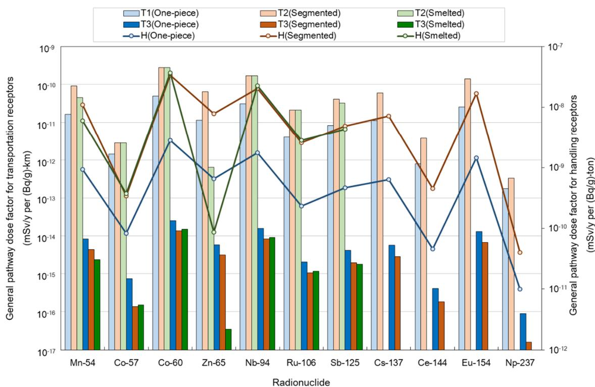
**Figure 4.** General pathway dose factor for each radionuclide and for each receptor, from T1 to T3 (read left Y axis) and H (read right Y axis), involved in the transportation of the steam generator as calculated in this study.
