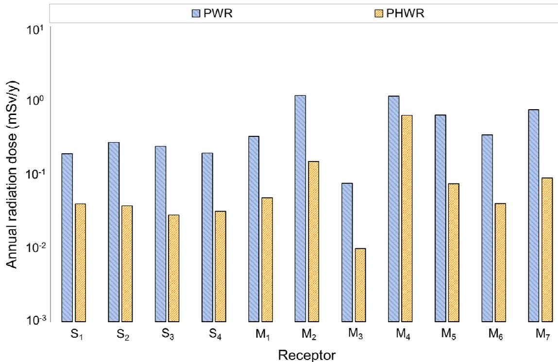
**Figure 5.** Radiation dose of receptors  $S_1$  to  $M_7$  involved in the processing of the PWR or PHWR steam generator calculated in the specific assessments.
