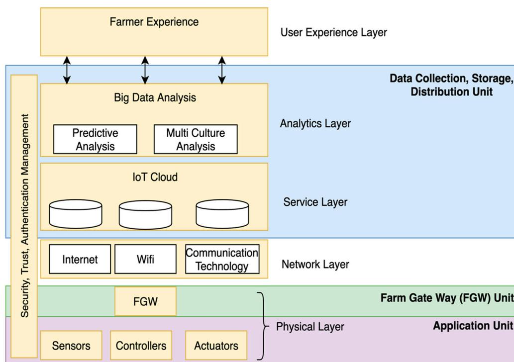
**Figure 1.** Internet of Things (IoT)-based agriculture and plant factory units framework (modified from [6]).
