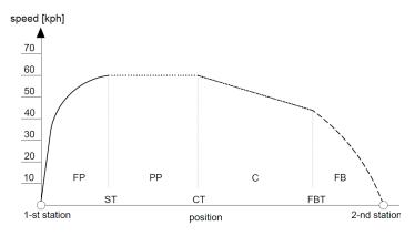
Figure 1. Optimal vehicle speed profile (source: [26]).
