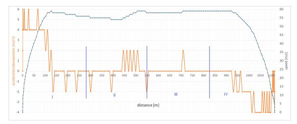
Figure 5. Train movement diagram (source: own elaboration).
