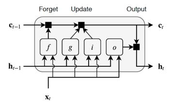
Figure 4. LSTM block structure (source: [36]).
