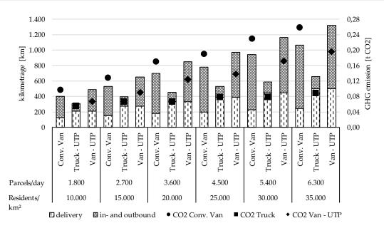
**Figure 3.** Kilometrage and greenhouse gas (GHG) emissions; comparison of conventional delivery and UTP strategy U-C with trucks and vans.
