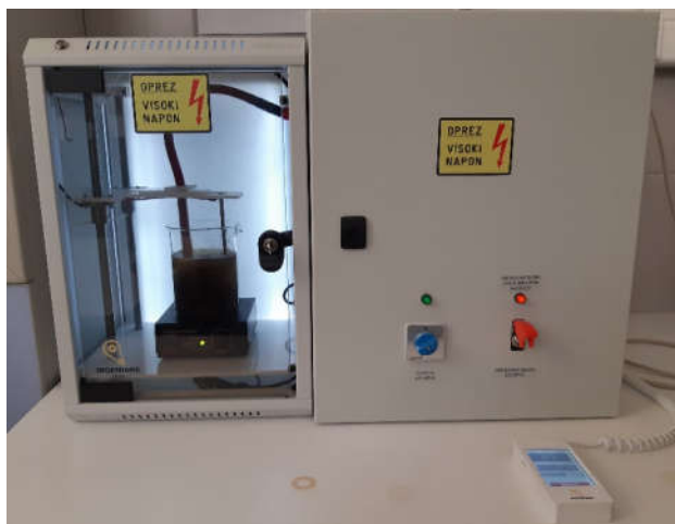
Figure 1. High voltage electrical discharge device.
