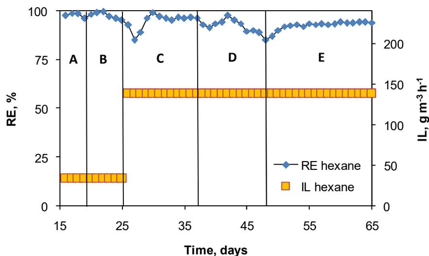
**Figure 3.** The course of the biotrickling filtration of hexane treated simultaneously with ethanol. (A)  $\theta = 1$ ; (B)  $\theta = 2$ ; (C)  $\theta = 0.5$ ; (D) ethanol starvation; (E)  $\theta = 0.25$ .
