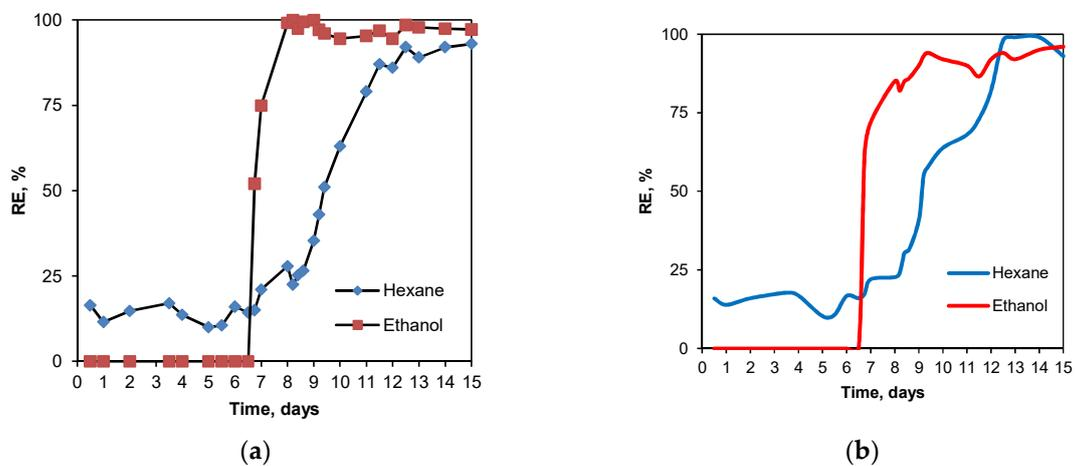
**Figure 1.** Biotrickling filter performance during the start-up period: introduction of hydrophilic ethanol on the sixth day of the process. Inlet loadings:  $34.5 \text{ g m}^{-3} \text{ h}^{-1}$  (hexane) and  $18.45 \text{ g m}^{-3} \text{ h}^{-1}$  (ethanol): (a) process control realized by gas chromatography; (b) process control by electronic nose.
