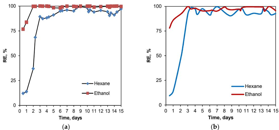
**Figure 2.** Biotrickling filter performance during the start-up period. Inlet loadings:  $34.5 \text{ g m}^{-3} \text{ h}^{-1}$  (hexane) and  $18.45 \text{ g m}^{-3} \text{ h}^{-1}$  (ethanol): (a) process control by gas chromatography; (b) process control by electronic nose.
