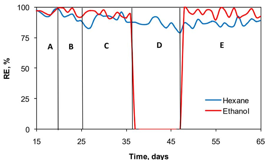
**Figure 5.** The course of biotrickling filtration of ethanol treated simultaneously with hexane. (A)  $\theta = 1$ ; (B)  $\theta = 2$ ; (C)  $\theta = 0.5$ ; (D) ethanol starvation; (E)  $\theta = 0.25$ . Process performance control using electronic nose.
