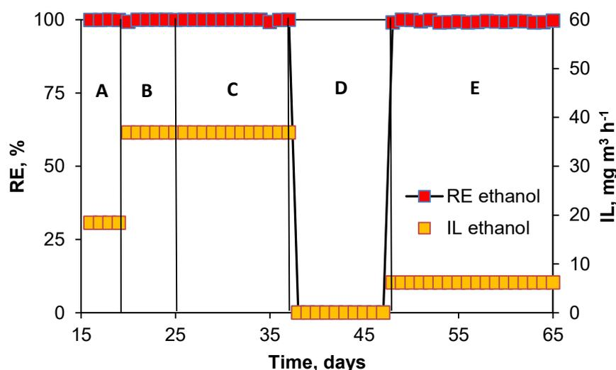
**Figure 4.** The course of biotrickling filtration of ethanol treated simultaneously with hexane. (A)  $\theta = 1$ ; (B)  $\theta = 2$ ; (C)  $\theta = 0.5$ ; (D) ethanol starvation; (E)  $\theta = 0.25$ .
