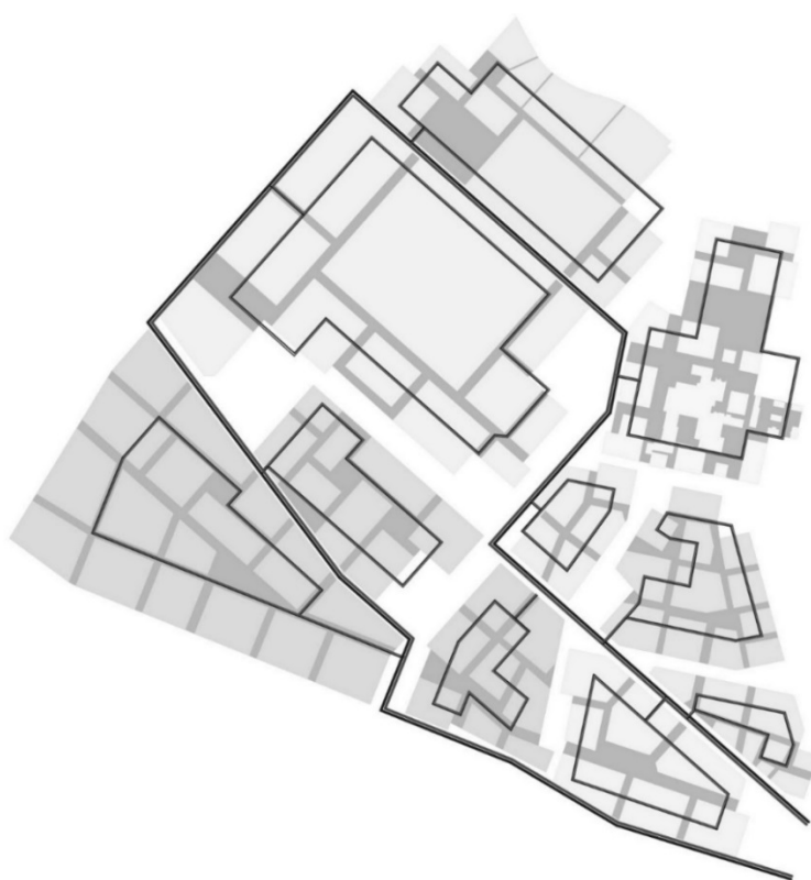
Figure 1. Energy communities formulate a regional system with a district heating system. Thick lines represent district heating, thin lines represent the local network of the integrated community energy system (ICES), and grey fields represent superblocs.
