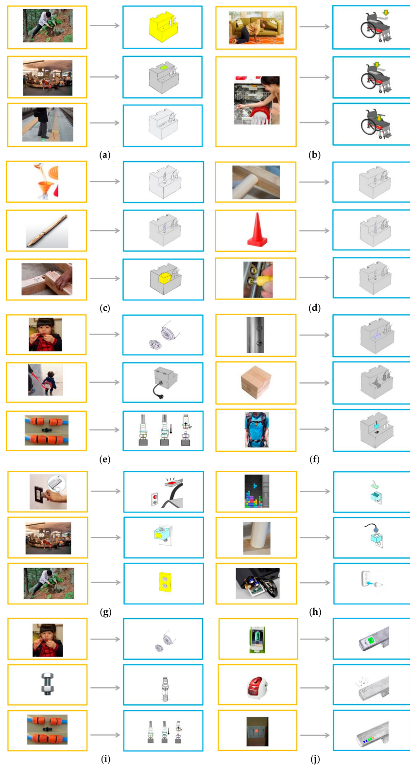
Figure 7. Affordance Features. (a) Find-ability (Find the Battery). (b) Access-ability (Find Location of the Adapter hole). (c) Align-ability (Align the Adapter and the Battery hole). (d) Insert-ability (Insert the Adapter). (e) Connect-ability (Connect the Adapter to the Battery). (f) Check-ability (Check Connection of the Battery). (g) Find-ability (Find the Outlet). (h) Insert-ability (Insert the Adapter plug to the Outlet). (i) Connect-ability (Connect the Adapter to the Outlet). (j) Check-ability (Check Connection of the Outlet).
