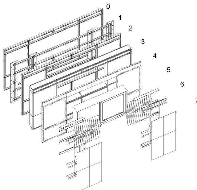
**Figure 11.** Enhanced building envelope system exemplary façade module. Each layer number is associated with the description provided in Table 5 below.
