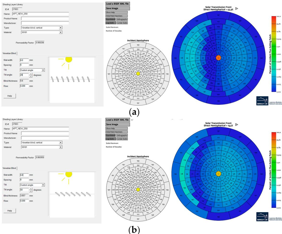
**Figure 15.** (Left) WINDOW-generated BSDLF-based shading position for (a) 20° orientation (2—slightly closed condition) and (b) 50° orientation (3—partially closed). (Right) BSDLF solar transmission hemispherical sky map for (a) 20° orientation (2—slightly closed condition) and (b) 50° orientation (3—partially closed), visualized with the Radiance-developed BSDLFviewer.
