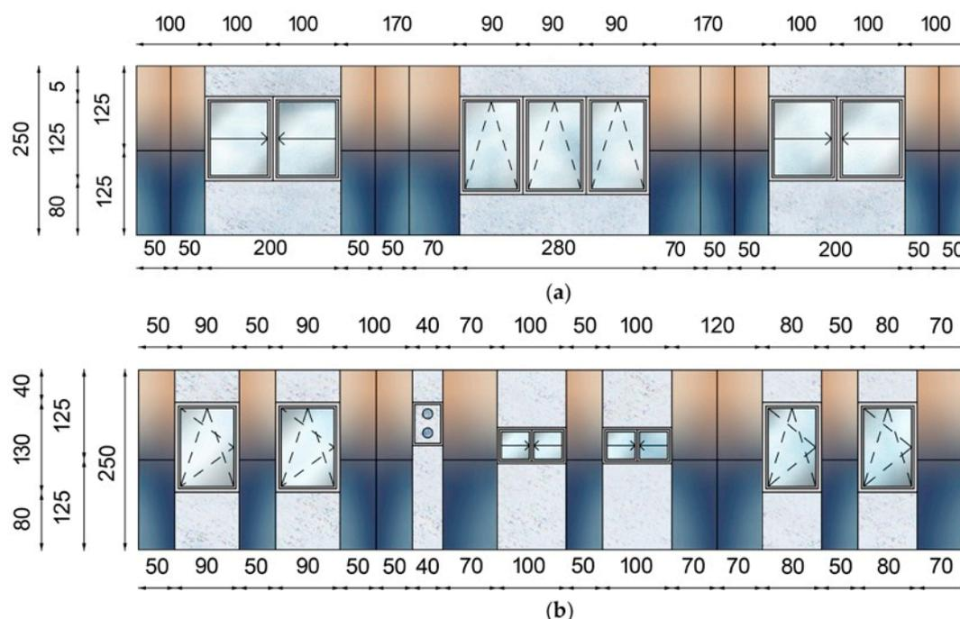
**Figure 12.** Enhanced building envelope system mounted on (a) south-oriented façade and (b) north-oriented façade (measures in cm).
