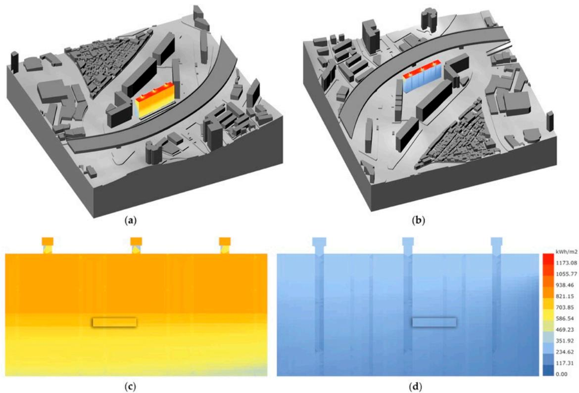
**Figure 7.** Annual cumulative solar radiation analysis of building 103: (a) Solar analysis with contextual shading for the south-oriented façade; (b) solar analysis with contextual shading for the north-oriented façade; (c) overview of cumulative annual solar radiation for the South-oriented façade and the reference apartment (marked surface); and (d) overview of cumulative annual solar radiation for the north-oriented façade and the reference apartment (marked surface).
