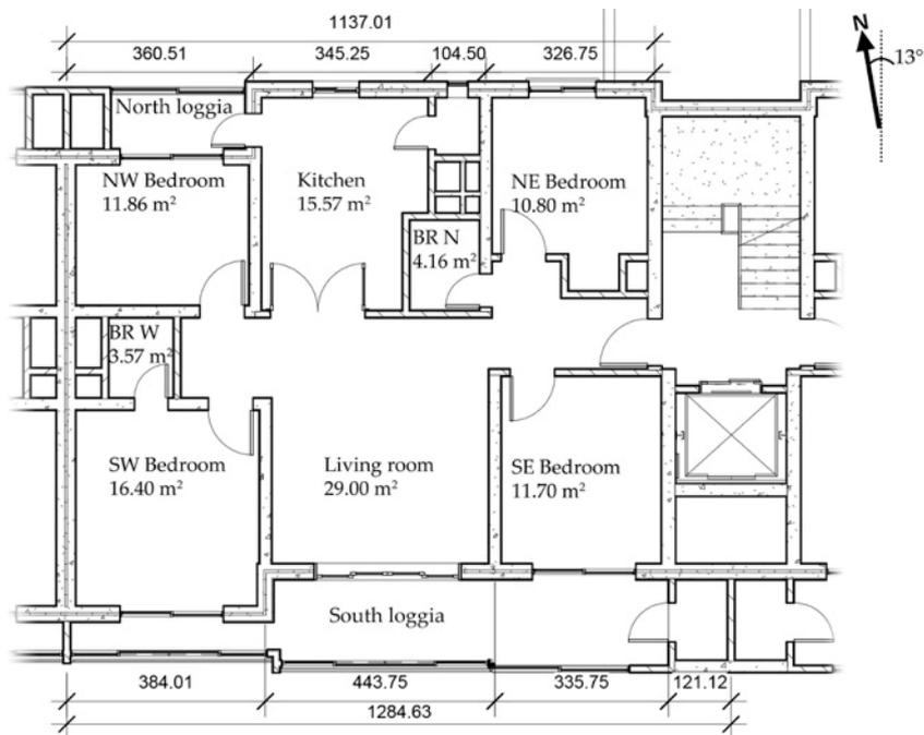
**Figure 4.** BIM reconstruction of the standard apartment unit in building 103 with indication of each room floor space (left apartment unit in the middle core—dimension annotations in cm).
