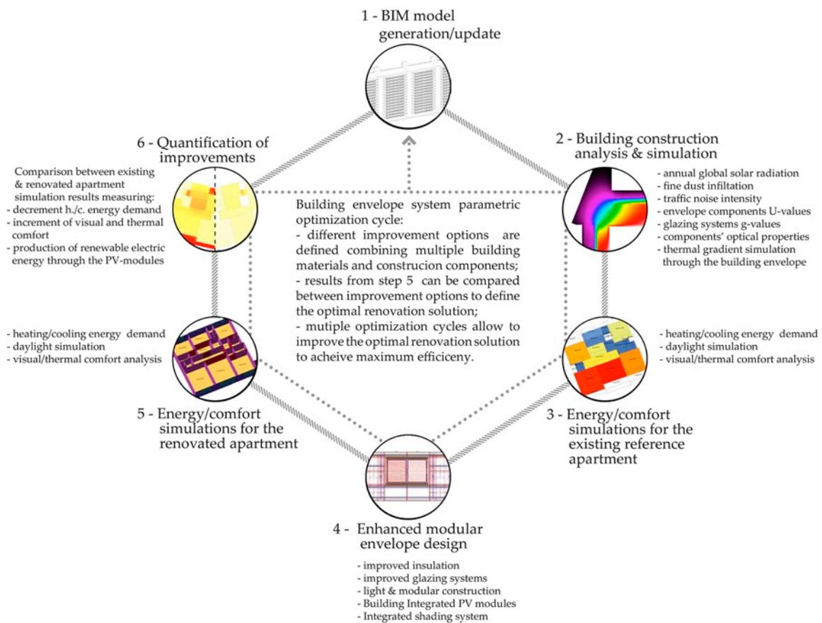
**Figure 2.** Overview of the Building Information Modeling (BIM)-parametric renovation framework utilized for the development of the sustainable renovation strategy for the exemplary apartment building. The framework is organized in one BIM-model generation/update and five recursive parametric optimization phases.
