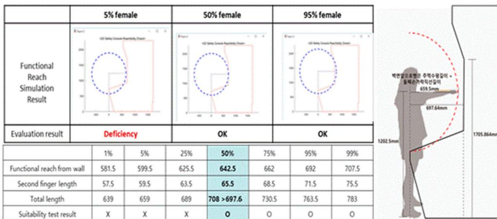
**Figure 13.** VR-based system simulation result showing human engineering deficiency for functional reach and suggested design change of the safety console. 5% female’s actual reach is deficient from 50% female (blue dashed).
