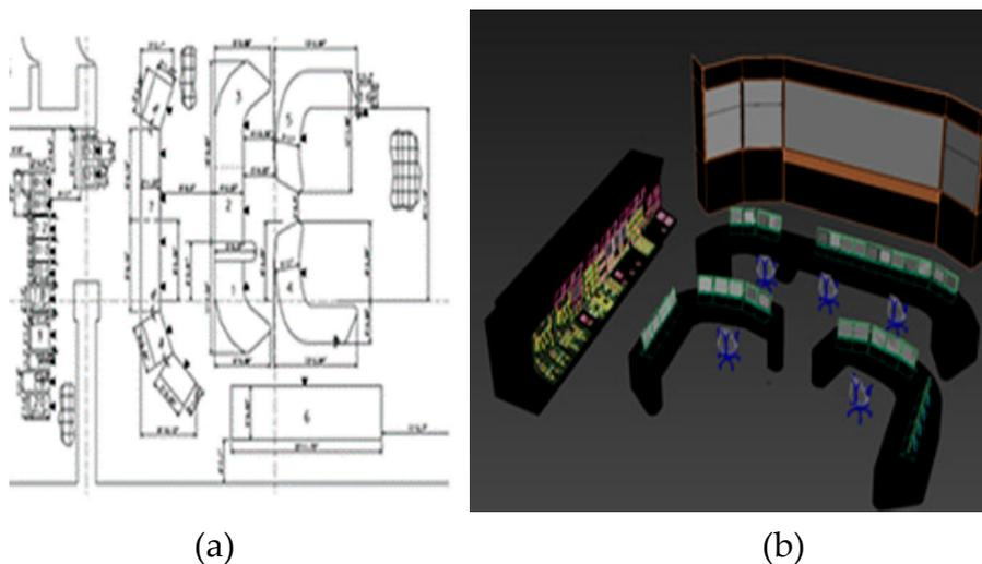
Figure 6. The implemented intelligent design review system (IDRS) virtual model: (a) 2D MCR drawings; (b) the implemented 3D MCR model.
