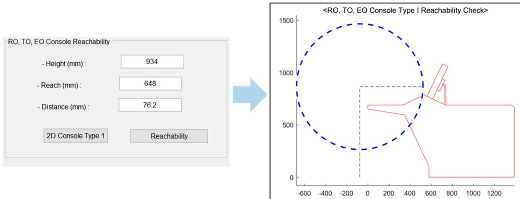
**Figure 12.** Design improvement result for console reachability check in the IDRS. The VR-based system proposed the monitor size change for better visual angle and comfort in the working environment (The y axis indicates heights and the x axis is the depth from the sitting point; unit: mm).
