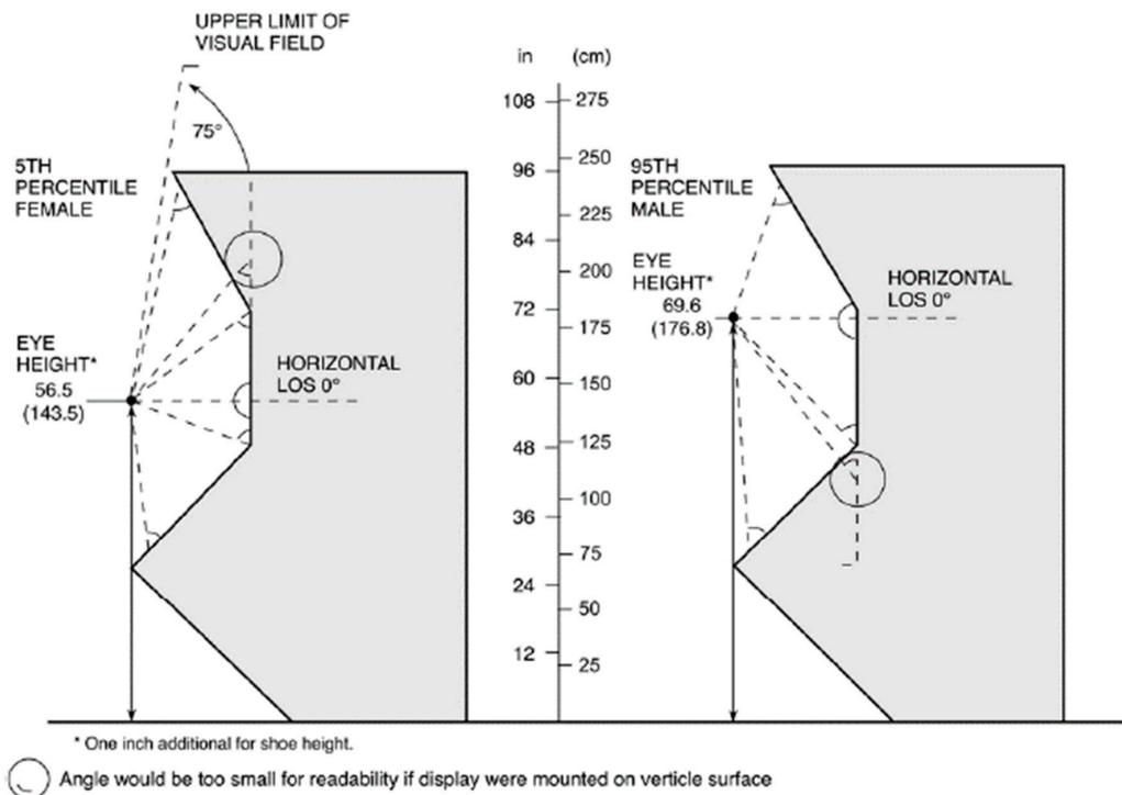
**Figure 2.** Display height and orientation relative to a standing user’s line of sight [25,26].
