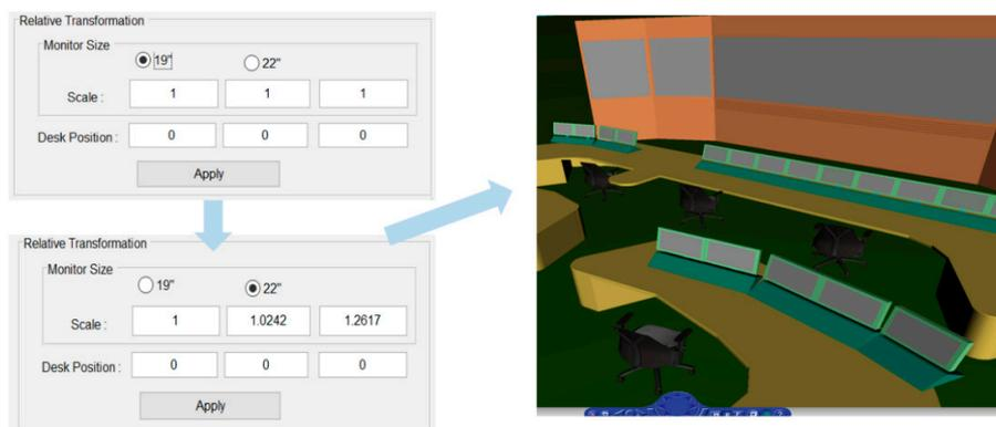
**Figure 8.** Parametric conversion process of each component in the MCR.
