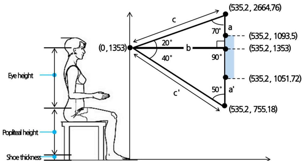
Figure 4. Sit-down console design computational model with anthropometric data usage (male 95<sup>th</sup> percentile of the 7th Korean Anthropometric Data Survey Report [8]).
