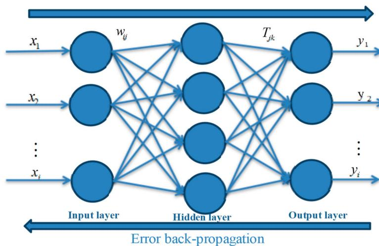
Figure 1. The structure of Three-Layer BP Neural Network.
