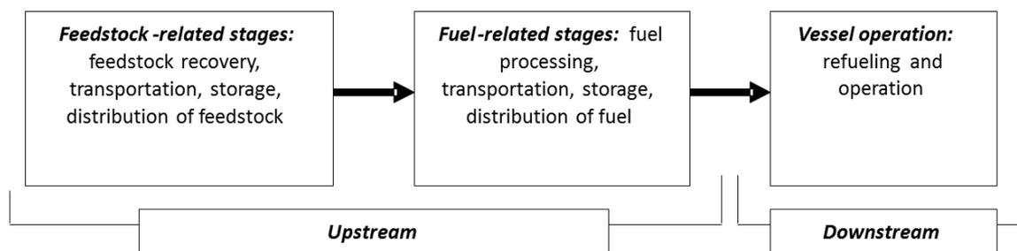
**Figure 1.** Components of a total fuel cycle analysis showing upstream (“well-to-tank”) and downstream (“tank-to-propeller”) activities [7].
