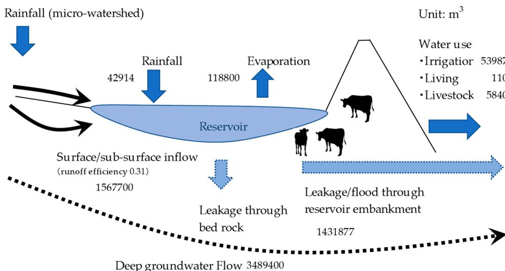
Figure 6. The water balance of the Adizaboy reservoir.
