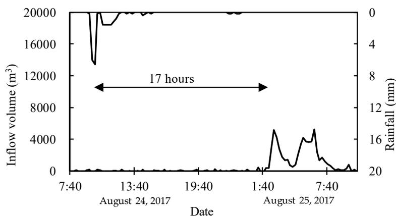
Figure 5. The hyetograph/hydrograph of the reservoir in the Adizaboy micro-watershed.
