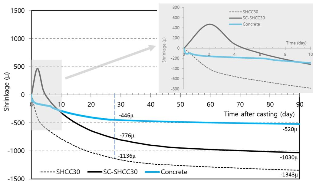
**Figure 2.** Shrinkage history of concrete and SHCC materials in a standard environment.
