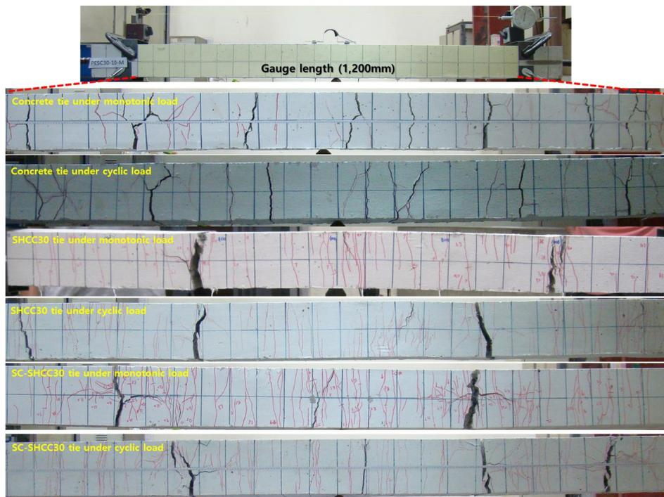
Figure 8. Failure modes of concrete and SHCC material tension ties.
