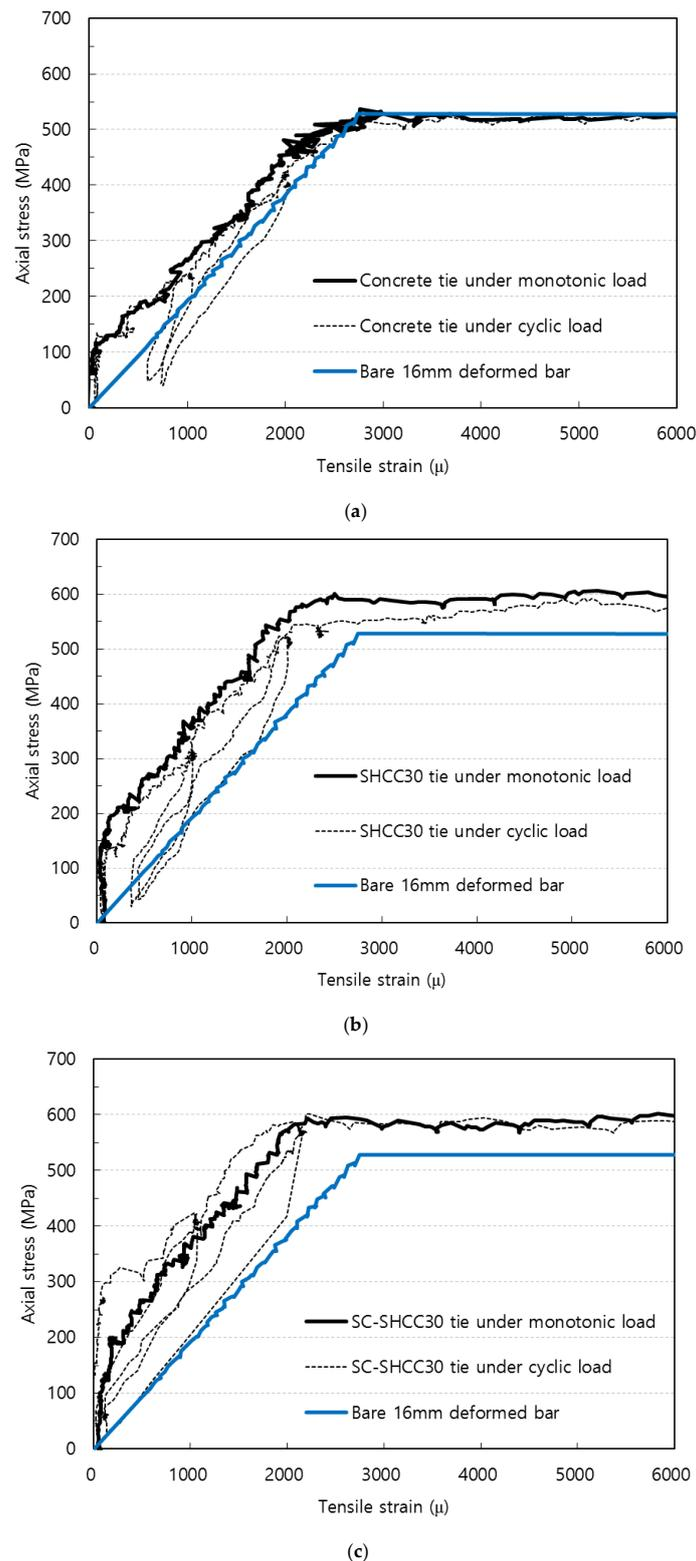
**Figure 6.** Axial stress versus strain curves of tension ties under monotonic and cyclic load. (a) Concrete tension ties; (b) SHCC30 tension ties; (c) SC-SHCC30 tension ties.
