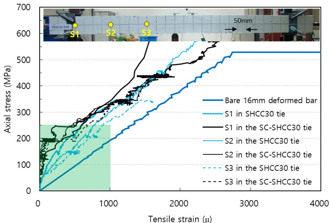
Figure 7. Axial stress versus local strain curves of rebar in ties under monotonic load.
