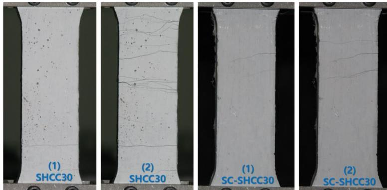
Figure 4. Tensile response (top) and cracking patterns (bottom) of SHCC dumbbell-shaped specimens.
