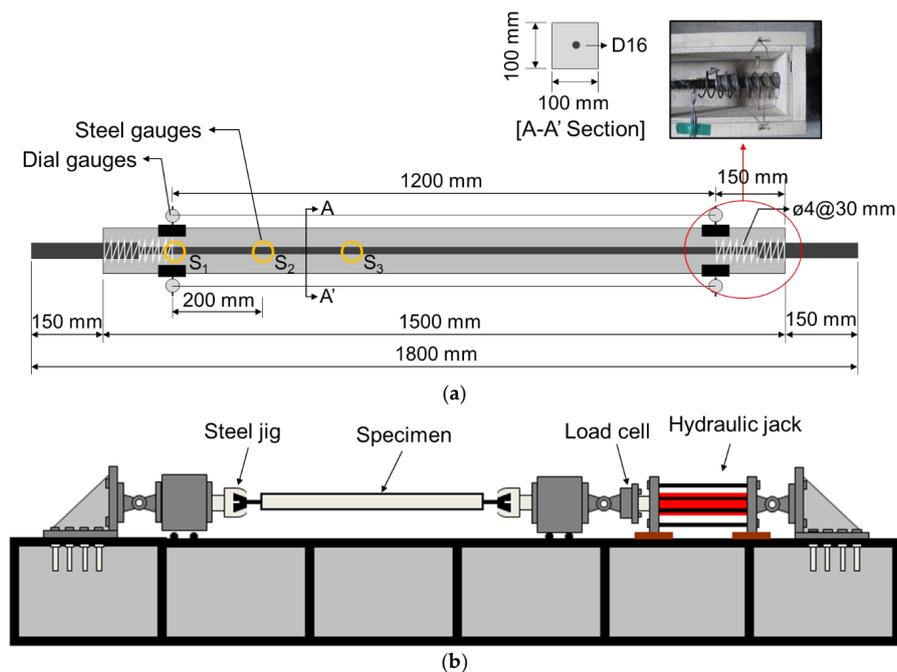
**Figure 1.** Specimen configuration and test setup on tension ties. (a) Configuration and dimensions; (b) Test set-up.
