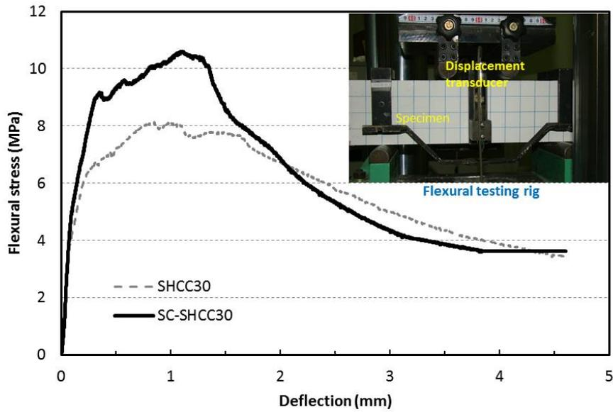
Figure 3. Flexural responses of SHCC prismatic specimens.
