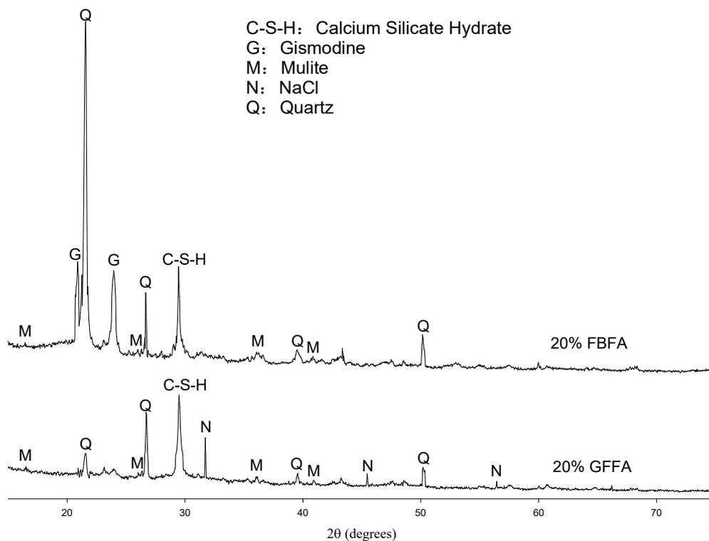
**Figure 4.** Results of XRD analyses for the new developed GFFA- and FBFA-containing bricks.
