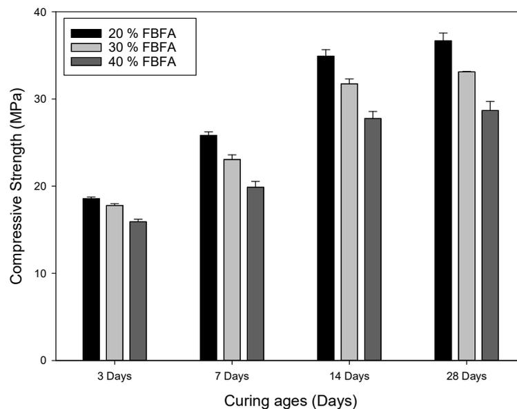
**Figure 2.** Compressive strength with different percentages of the FBFA in the alkali-activated bricks.
