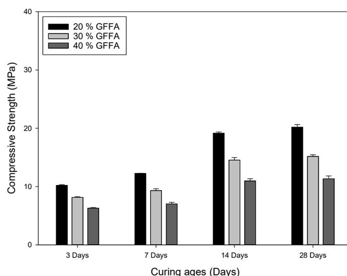
**Figure 1.** Compressive strength with different percentages of the GFFA in the alkali-activated bricks.
