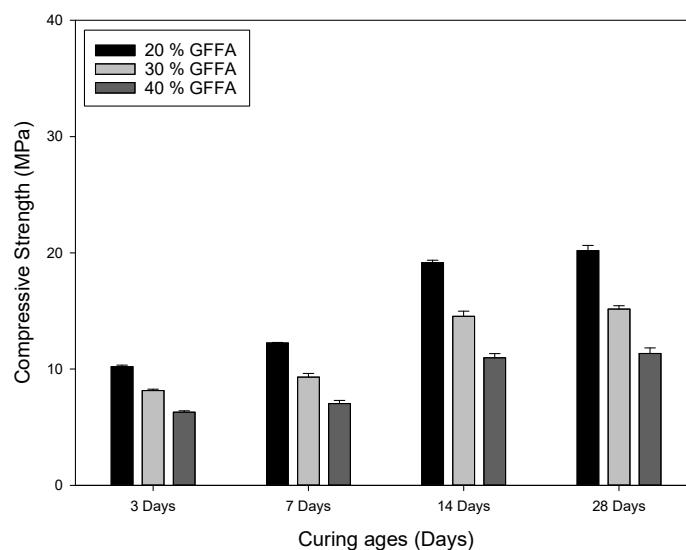
**Figure 1.** Compressive strength with different percentages of the GFFA in the alkali-activated bricks.
