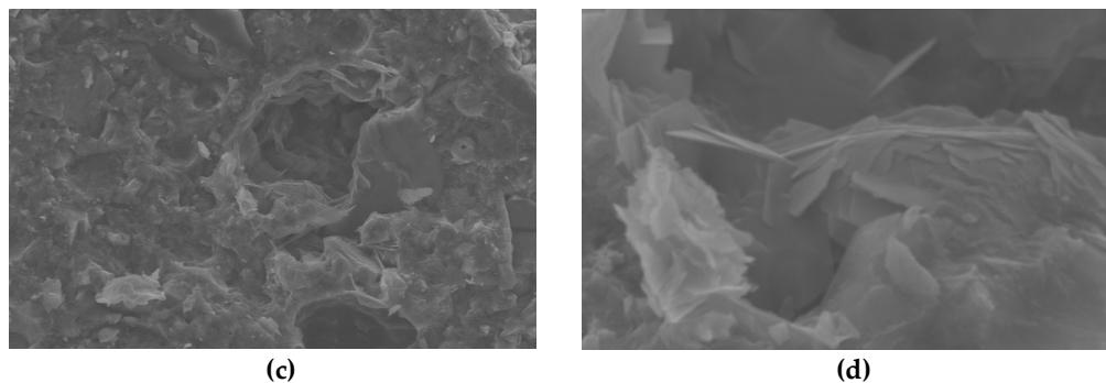
**Figure 3.** (a) Alkali-activated brick containing 20% GFFA, 1000-fold magnification; (b) Alkali-activated brick containing 20% GFFA, 6000-fold magnification; (c) Alkali-activated brick containing 20% FBFA, 1000-fold magnification; (d) Alkali-activated brick containing 20% FBFA, 6000-fold magnification.
