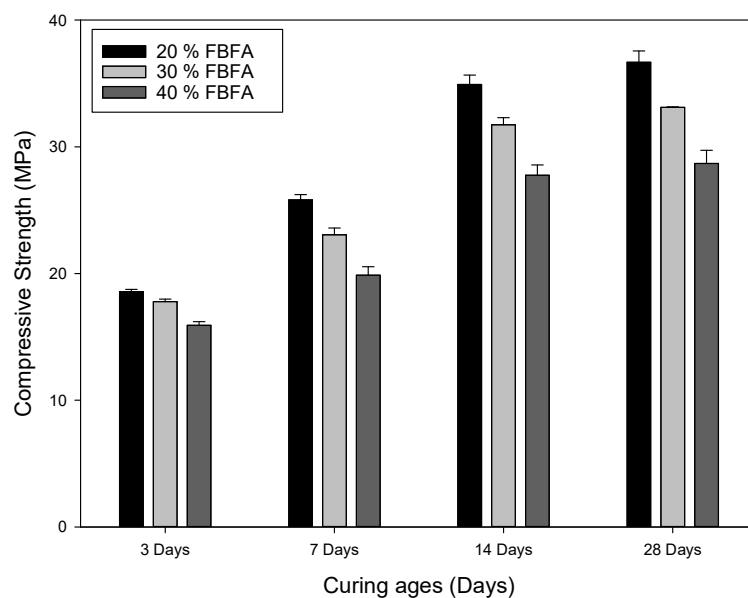
**Figure 2.** Compressive strength with different percentages of the FBFA in the alkali-activated bricks.
