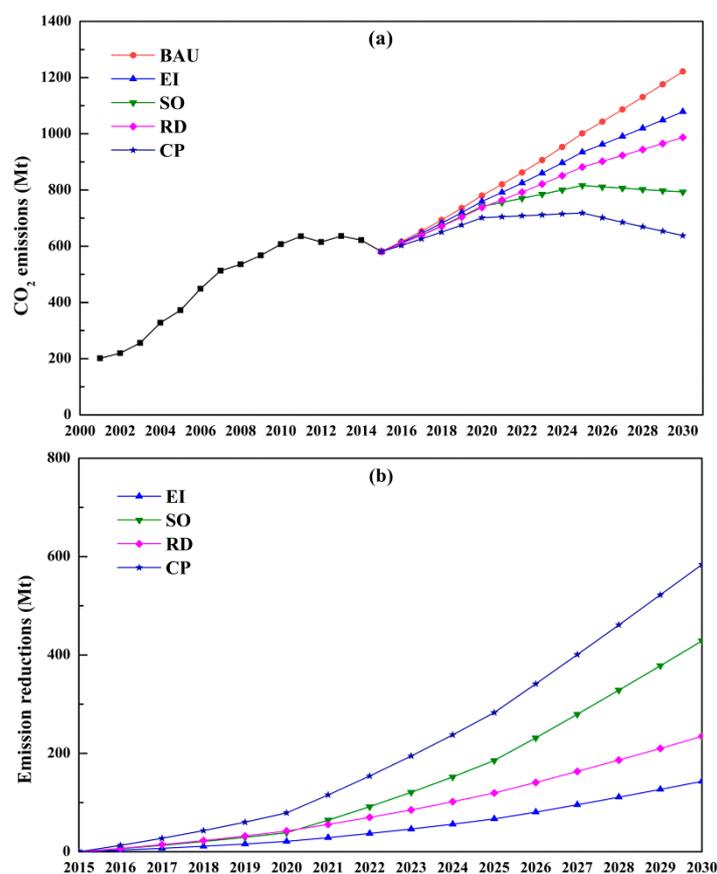
**Figure 8.** Industrial energy-related CO<sub>2</sub> emissions and mitigation potential: (a) Historical and future CO<sub>2</sub> emission trends over 2001–2030 under five scenarios and (b) CO<sub>2</sub> mitigation potentials over 2015–2030 under four scenarios.
