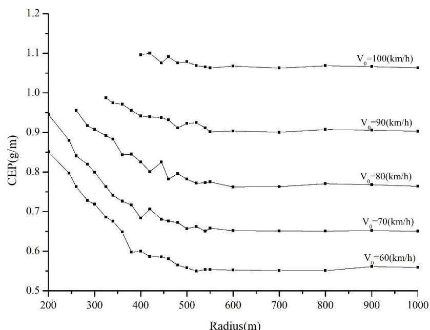
**Figure 4.** The carbon emission rate of field test on circular curves.
