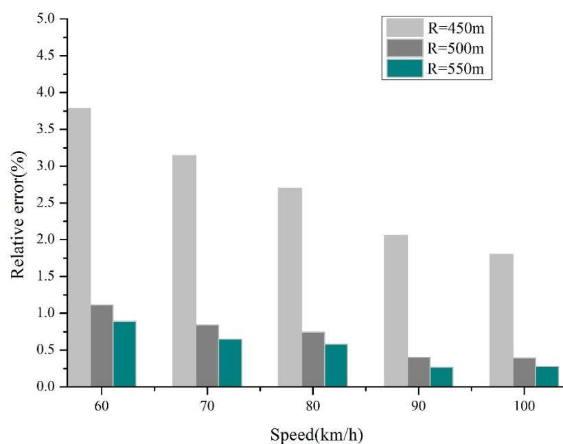
**Figure 6.** Partial relative error of carbon emissions in simulated scenarios.
