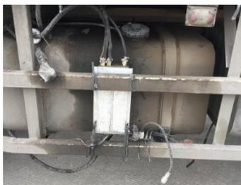
**Figure 1.** Fuel-consumption instrument used in field experiments.
