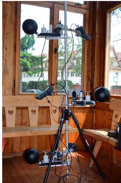
**Figure 9.** Test device for measuring thermal comfort.
