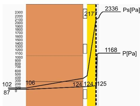
**Figure 8.** An example of a solution of how to insulate a historic building from the inside (authors' own calculations and image).
