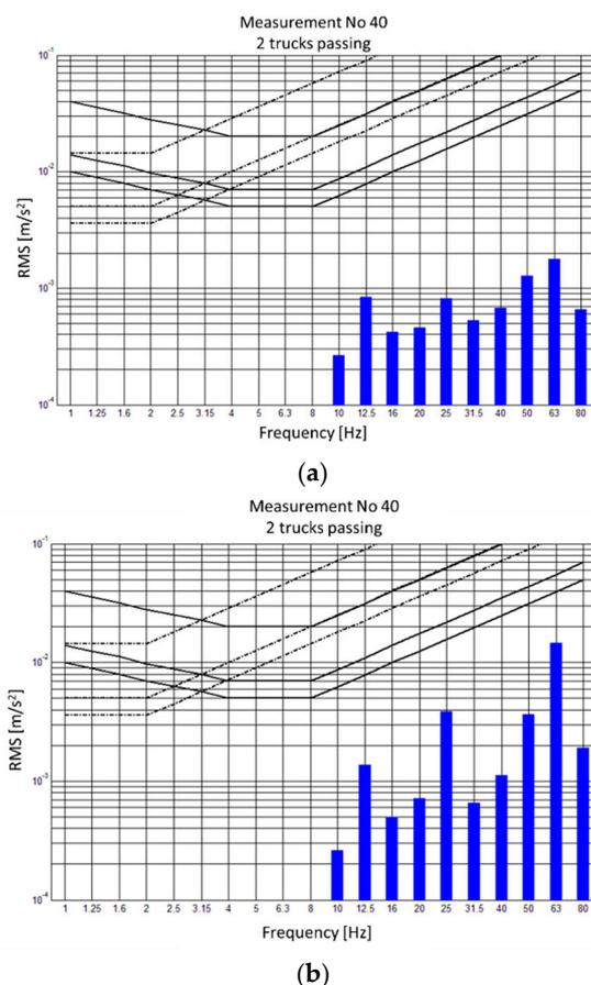
**Figure 15.** RMS analysis of measurement no. 40: (a) in the hall, and (b) in the guest room.
