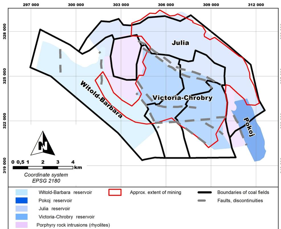
**Figure 3.** Borders of the WHCB mining areas with regard to the boundaries of underground water reservoirs. Local tectonic faults served as natural borders between the Julia and Victoria-Chrobry reservoirs and also between the Victoria-Chrobry and Witold-Barbara reservoirs.
