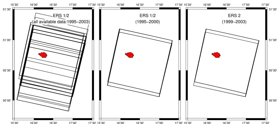
**Figure 6.** Selection of SAR data from ERS 1/2. The red polygon corresponds to the borders of the WHCB mining areas. The left-hand side of the figure shows the spatial distribution of SAR data from the analyzed Path 308, for the 1995–2010 period, a total of 147 images. It is interesting to observe the scale of image shift in the E-W direction, which is maximally 11 km. The middle part of the figure shows selected images for the 1995–2000 period and the right-hand side for the 1999–2002 period.
