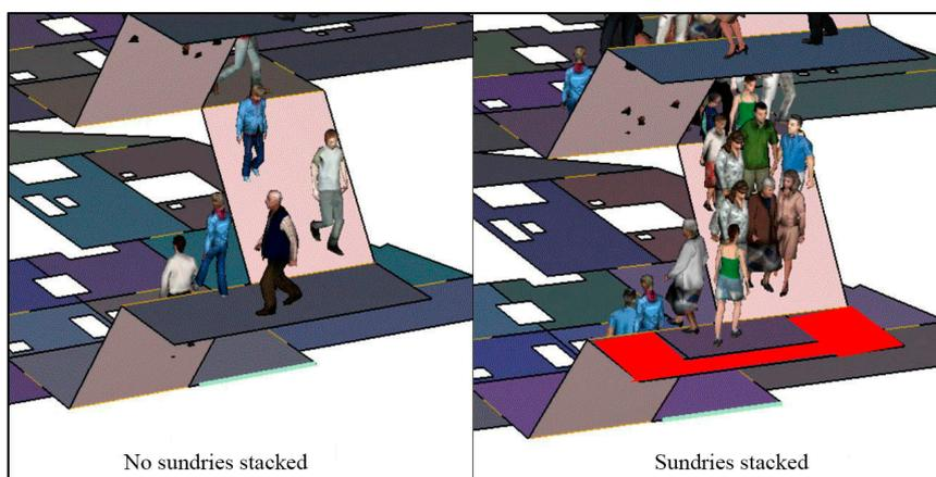
**Figure 13.** A contrastive case whether sundries exits or not in stairways between the 1st and 2nd floor (the red part represents stacked sundries).
