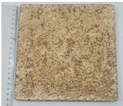
**Figure 10.** Slab measuring  $200 \times 200$  mm with 60% load of rubber in gold color with a differentiated surface.
