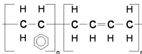
Figure 4. Chemical structure of styrene butadiene rubber (SBR).
