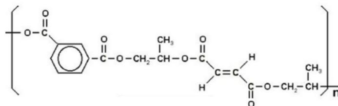
Figure 5. Isophthalic polyester resin chemical structure.
