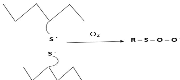
**Figure 6.** Opening of sulfur crosslinking and the action of oxygen in the environment.
