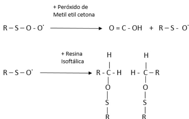
**Figure 7.** Reaction of the free radical of SBR with methyl ethyl ketone peroxide and isophthalic resin.
