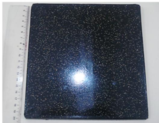
**Figure 8.** Slab measuring 200 × 200 mm with 60% ELTs in black color.
