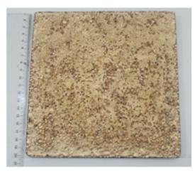
Figure 10. Slab measuring 200 × 200 mm with 60% load of rubber in gold color with a differentiated surface.
