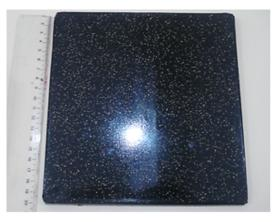
**Figure 8.** Slab measuring  $200 \times 200$  mm with 60% ELTs in black color.
