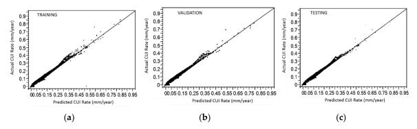
**Figure 6.** Actual vs. predicted corrosion rate in millimeters per year for a neural network. (**a**) Training, (**b**) Validation, and (**c**) Testing.
