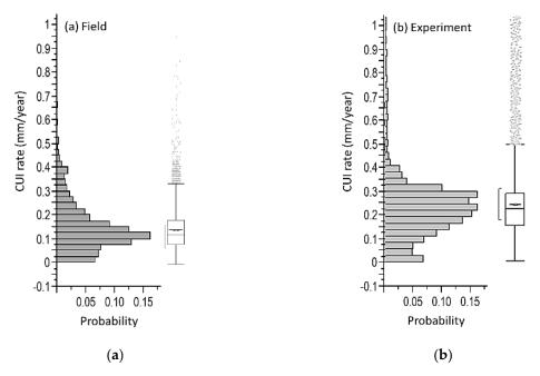
Figure 4. Distributions of simulated CUI rate (mm/year) from (a) field data, (b) experimental data.
