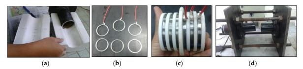
**Figure 2.** The initial phase of the experiment (**a**) Preparation of insulation material; (**b**) The corrosion under insulation (CUI) cell mock piping with blind flanges; (**c**) The ring specimens after surface finishing; (**d**) Preparation of the carbon steel ring specimens and a Teflon spacer.
