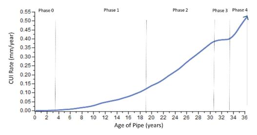
**Figure 8.** Relationship of the CUI rate and elapsed time in corrosion phases based on combined data input from field and experiment.
