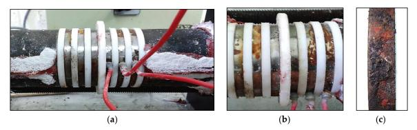
**Figure 5.** CUI rings specimens (**a**) condition after test completed and insulation dismantled, (**b**) a close up of the rings after the CUI test was completed, (**c**) close up of the ring surface with corrosion.
