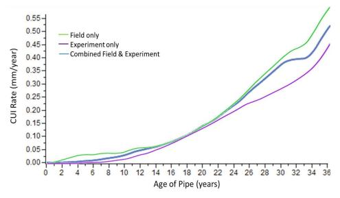
**Figure 7.** Comparison of CUI rate model developed based on single type input (Field only and Experiment only) with combined data input (Combined Field and Experiment).
