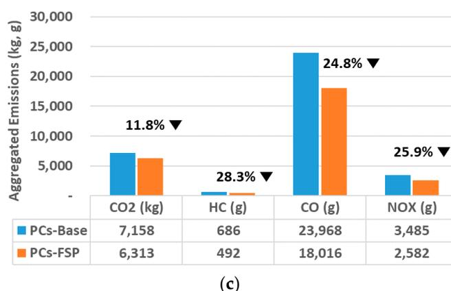
**Figure 3.** System-wide impacts of FSP on fuel consumption and emissions. Note: (a) Aggregated fuel consumption comparison; (b) comparison of emissions at  $V/C = 0.5$ ; (c) comparison of emissions at  $V/C = 0.85$ .
