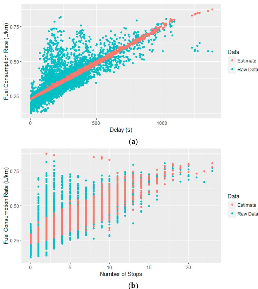
**Figure 5.** Scatter plot of fuel consumption rates and estimated fuel consumption rates Note: (a) Delay versus fuel consumption rate; (b) number of stops versus fuel consumption rate.
