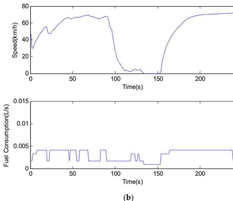
**Figure 2.** Trip comparison of normal truck (NT) and connected truck (CT). Note: (a) Sample trip of NT, Scenario-3; (b) sample trip of CT, Scenario-4.
